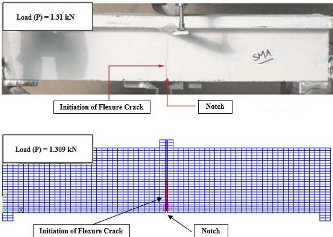
Figure 9. Initiation of flexural crack in the experimental and FE Simulation during 1<sup>st</sup> cycle
