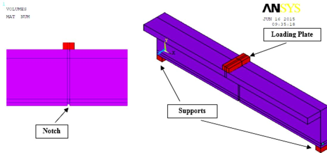
Figure 4. Finite element model of the SMA reinforced T-Beam in ANSYS
