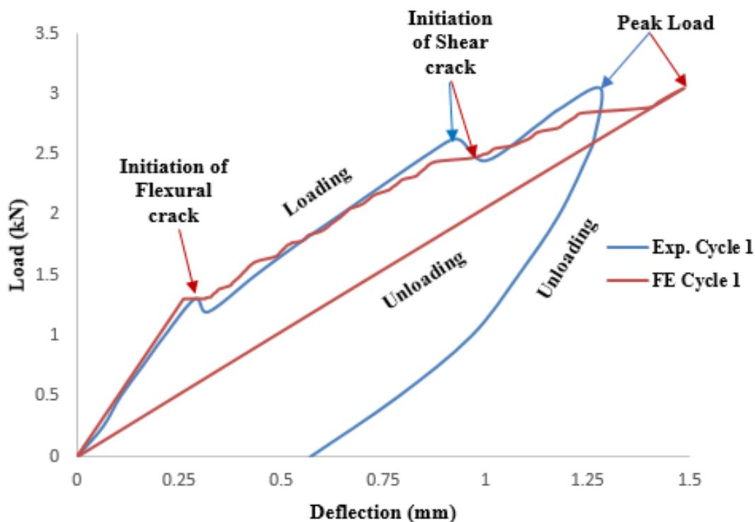
Figure 6. Load versus deflection between FE simulations and experimental for 1<sup>st</sup> cycle
