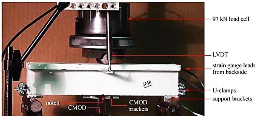
Figure 2. Experimental loading setup and support conditions (Zafar and Andrawes (2013))
