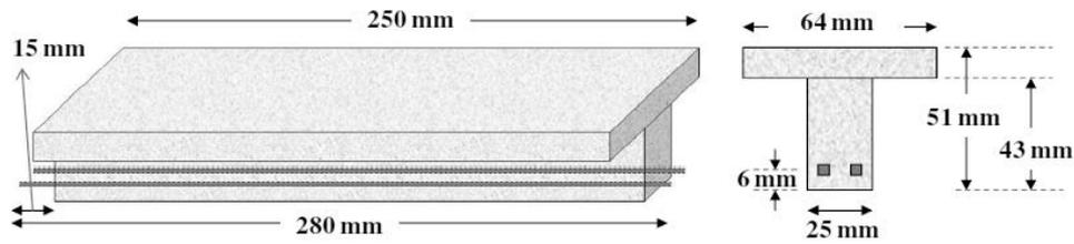
Figure 1. Cross sectional dimensions of T-beam tested (Zafar and Andrawes (2013))
