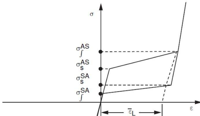
Figure 3. Idealized stress-strain diagram of superelastic SMA ANSYS
