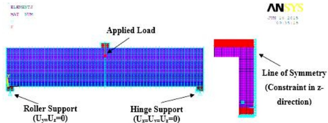
Figure 5. Boundary conditions and load applied
