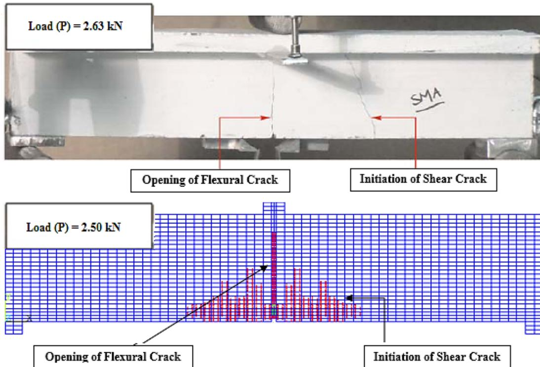
Figure 10. Initiation of shear crack in the experimental and FE simulation during 1<sup>st</sup> cycle
