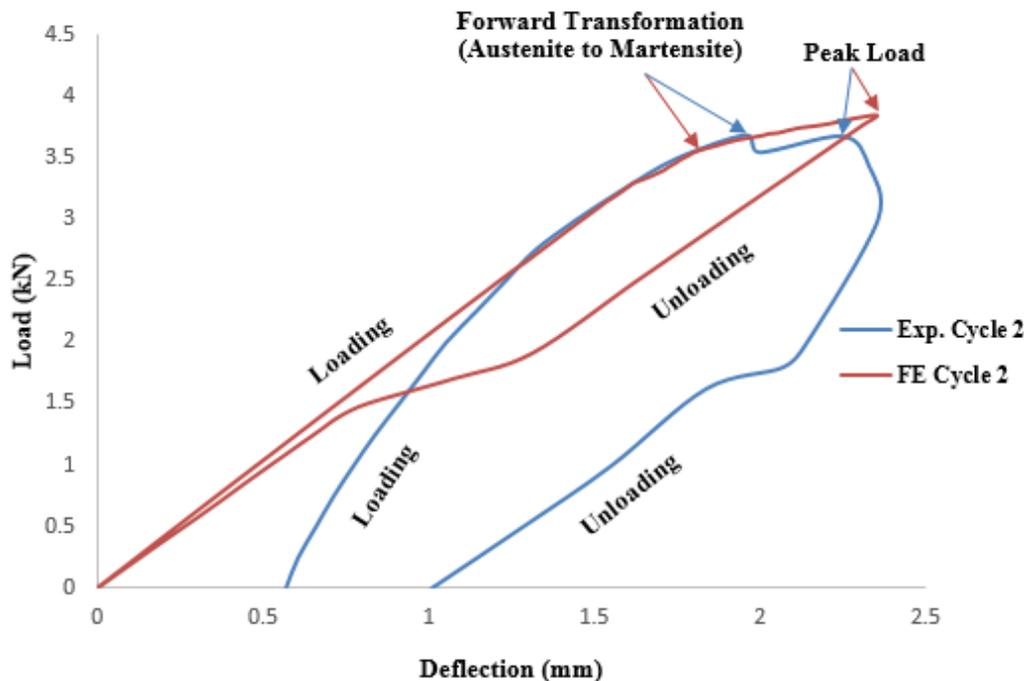
Figure 7. Load versus deflection between FE simulations and experimental for 2<sup>nd</sup> cycle
