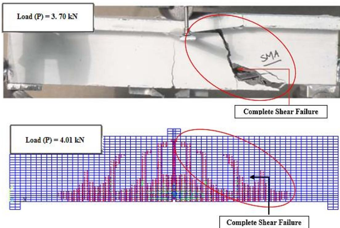
Figure 11. Complete Shear Failure in experimental and FE simulation at final stage
