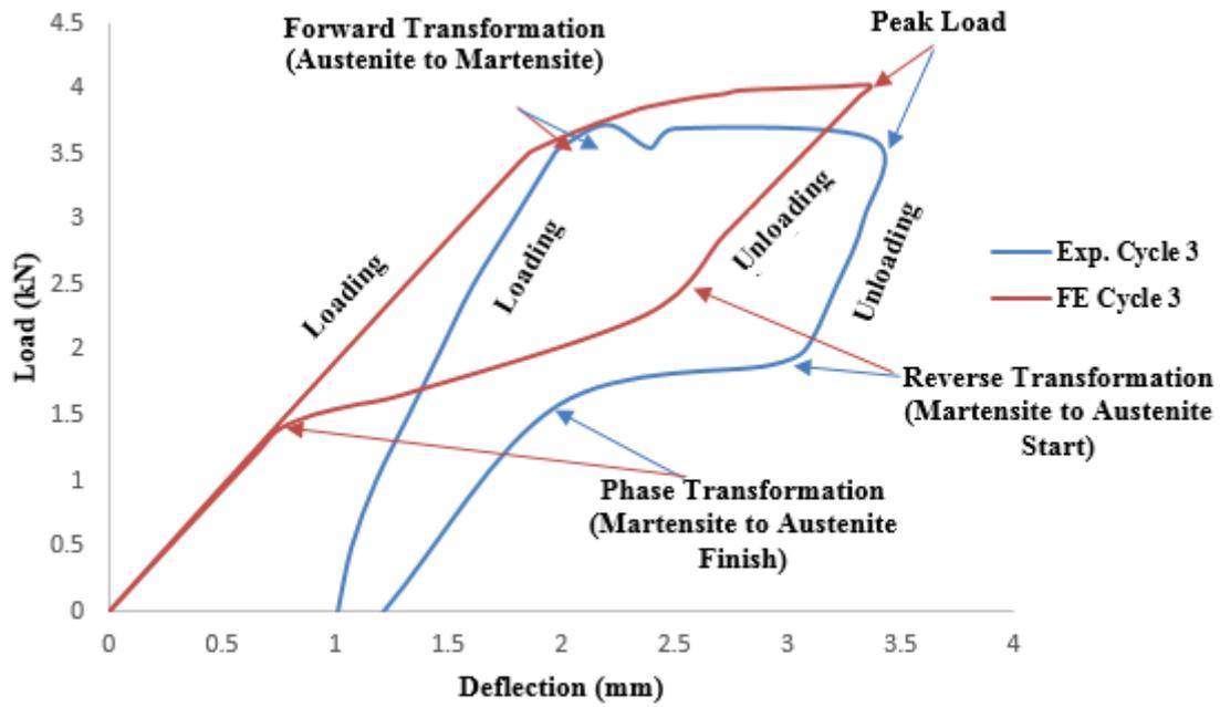
Figure 8. Load versus deflection between FE simulations and experimental for 3<sup>rd</sup> cycle
