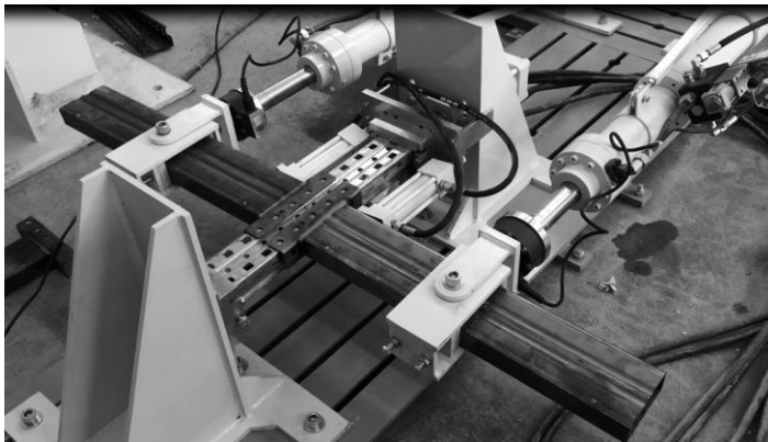
Figure 2. Experimental setup for cyclic testing of beam-to-column connections
