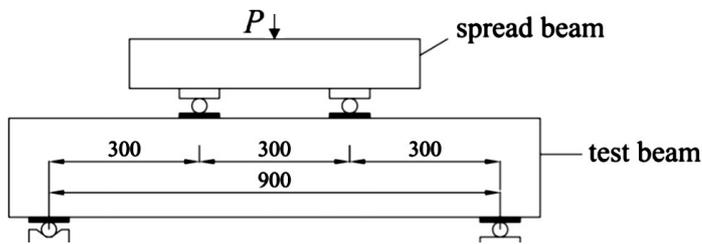
Figure 3. Beam test setup used by Lin et al (2013).
