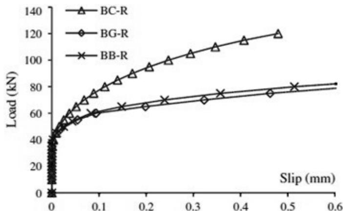
Figure 4. Load-slip relationships of concrete beams reinforced with different types of FRP rebars with ribbed surfaces (C - carbon, G - glass and B - basalt; Lin et al, 2013).
