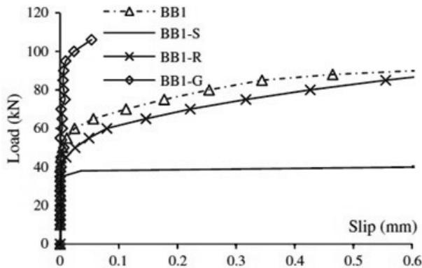
Figure 1. Load–slip relationships of BFRP reinforced concrete beams with different rebar surfaces (BB1 - wrapped, BB1-S - smooth, BB1-R - ribbed and BB1-G - grain-covered; Lin et al, 2013).
