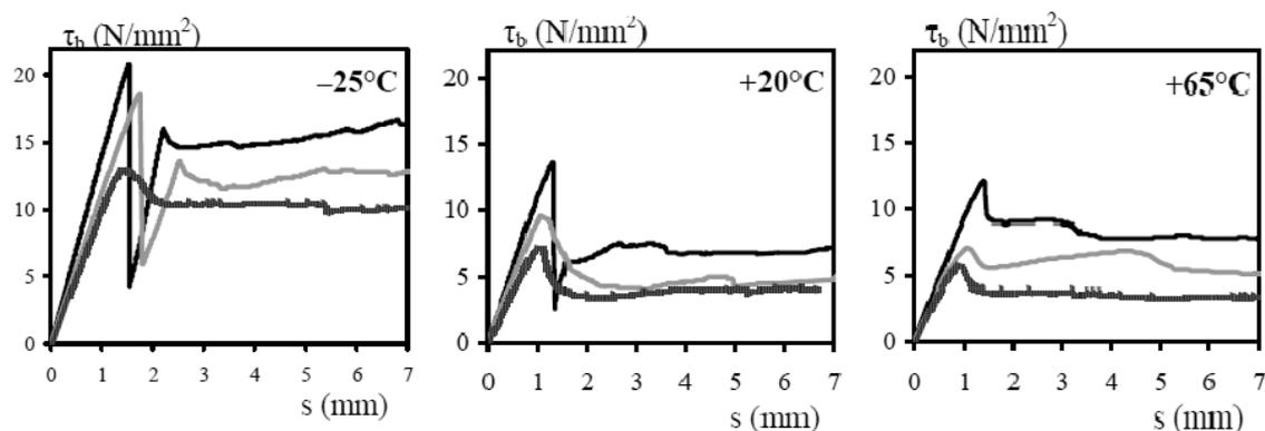
Figure 5. Testing temperature and typical bond stress ( $\tau_b$ ) vs. slip ( $s$ ) diagrams during static pull-out testing for sand coated CFRP wires. Three different concrete grades were studied (Borosnyói, 2015).
