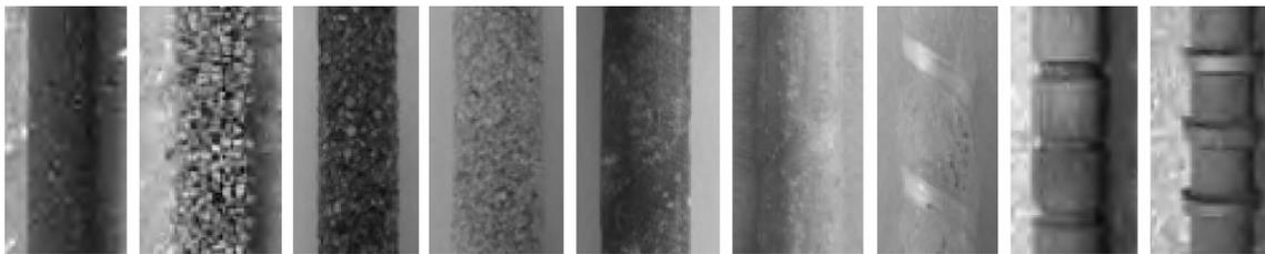
Figure 2. FRP bars with different surface characteristics. From left to right: plain surface; three different sand coated surface; texture surface; helical wrapping; helical wrapping and sand coated; two different indented surfaces (Al-Mahmoud et al., 2007; Baena et al., 2010).
