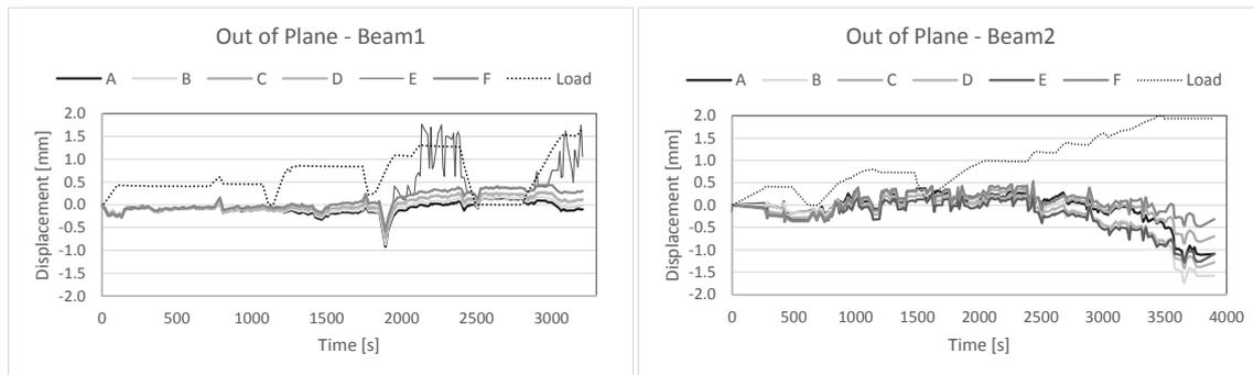
Figure 3. Out of plane displacement for Beam1 (left) and Beam2 (right).
