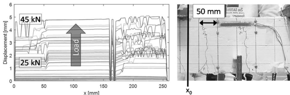
Figure 5. Beam1: horizontal displacement of for increasing load levels (left) and crack pattern (right).
