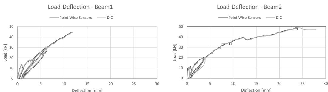
Figure 4. Load-deflection curves for Beam1 (left) and Beam2 (right).
