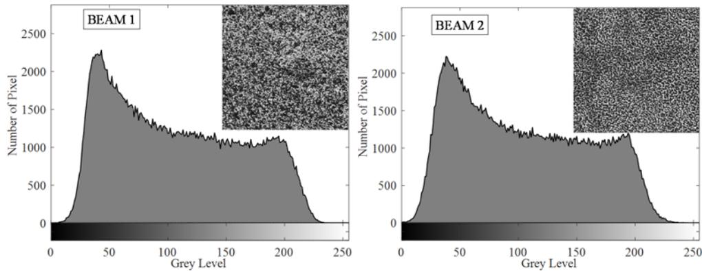
Figure 2. Speckle patterns and grey level histograms for a representative region of the two beams.
