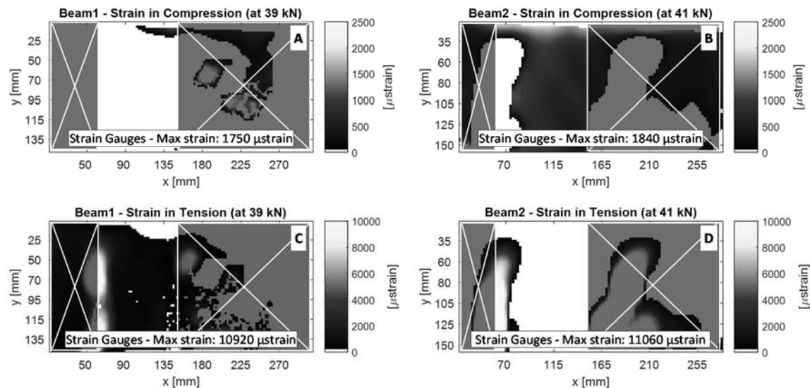
Figure 6. Full-field strains estimated with DIC for Beam1 (A and C) and Beam2 (B and D)
