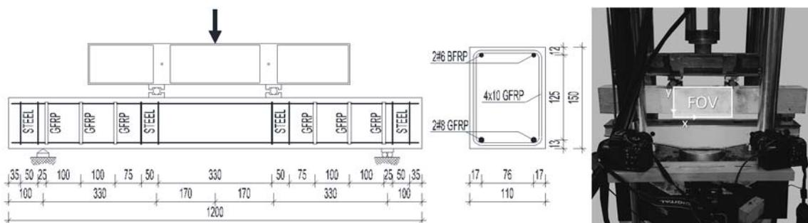
Figure 1. Test setup and internal reinforcement of the GFRP RC beams (left) and 3D-DIC test setup (right).
