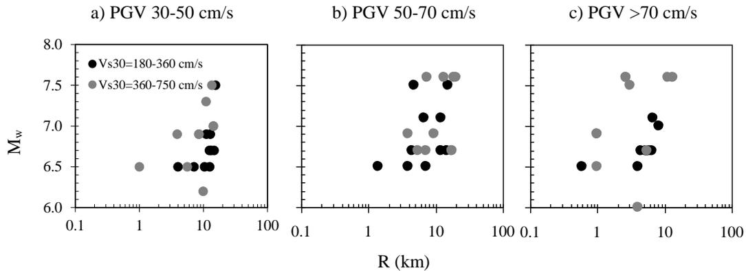
Figure 3. Closest distance to fault rupture ( $R$ ) versus magnitude ( $M_w$ ) for selected ground motions as a function of both site classification and PGV.
