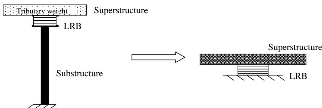
Figure 1. Idealization for seismic isolated bridge model.
