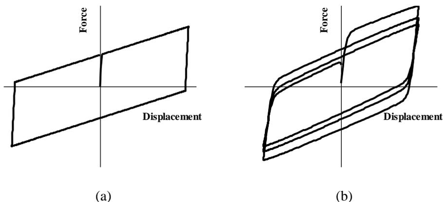
Figure 2. (a) Non-deteriorating and (b) deteriorating hysteretic force-deformation relationship for LRB.
