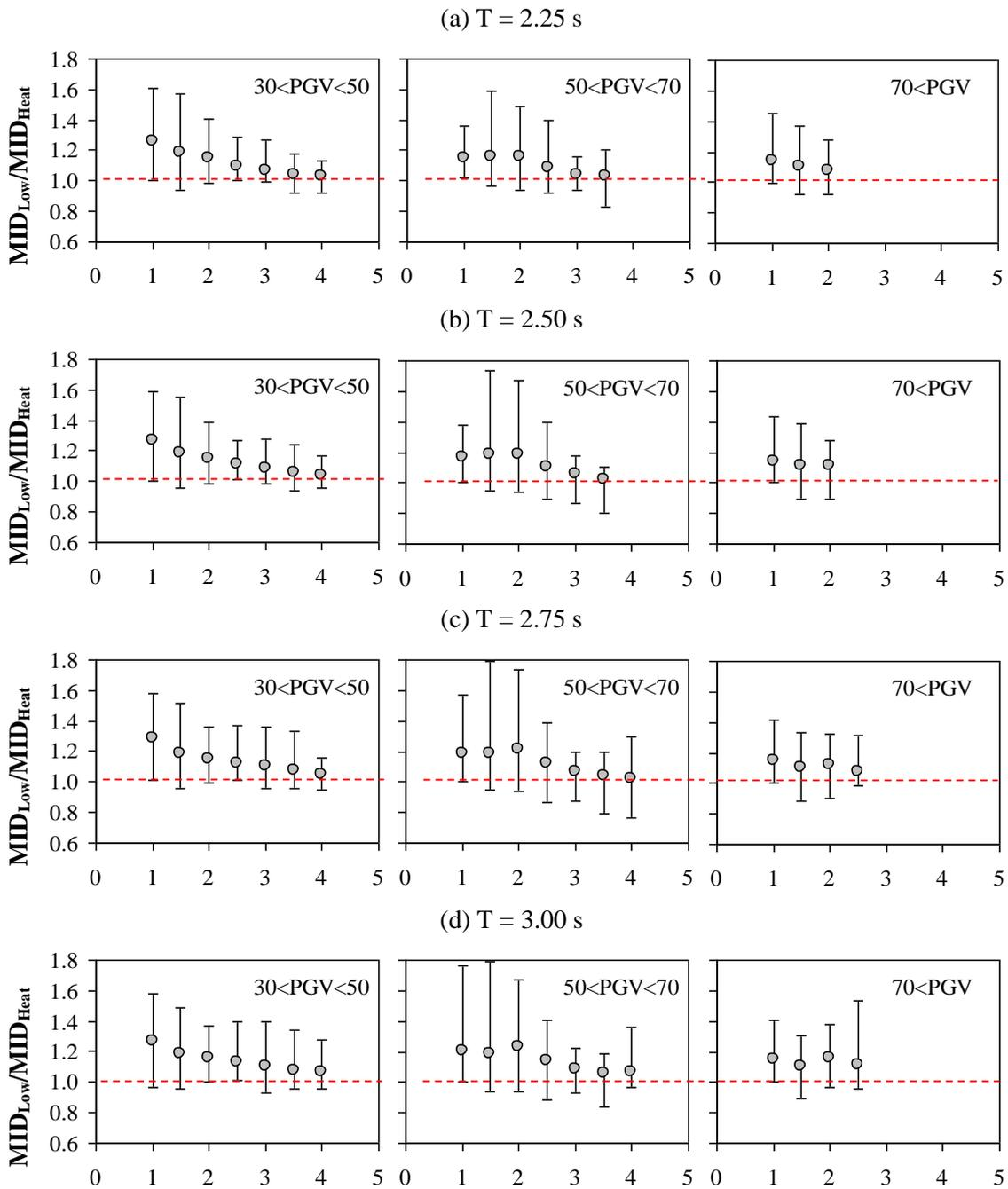
Figure 4. Variations of mean  $MID_{Low}/MID_{Heat}$  ratios for different PGV values and isolation periods.
