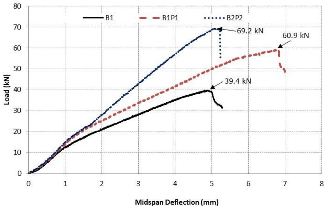
Figure 2. Load vs. midspan deflection for all tested specimens
