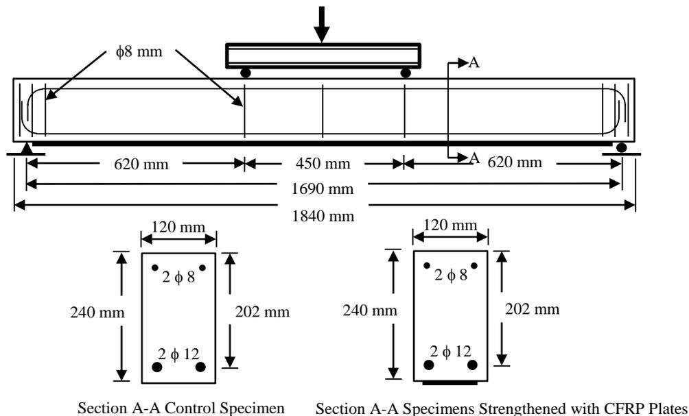
Figure 1. Specimens details and test setup
