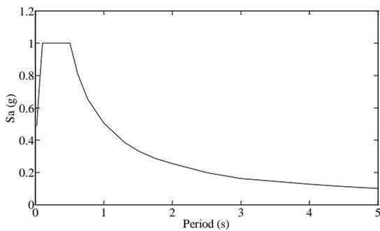
Figure 2. Design earthquake spectrum
