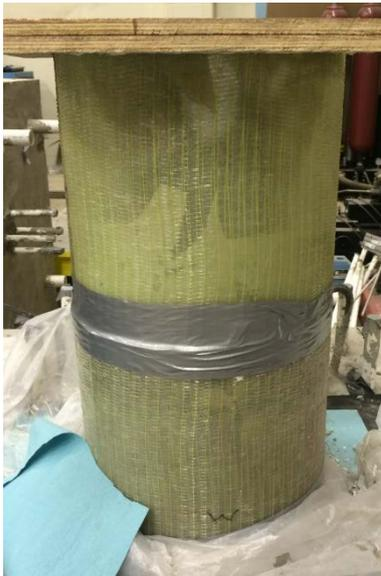
Figure 3. Match-casting of the column
