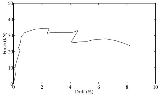
Figure 5. Dynamic backbone curve
