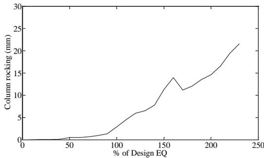
Figure 8. Rocking response of the column along the tests
