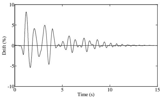
Figure 7. Response history of drift at 250% of the design earthquake
