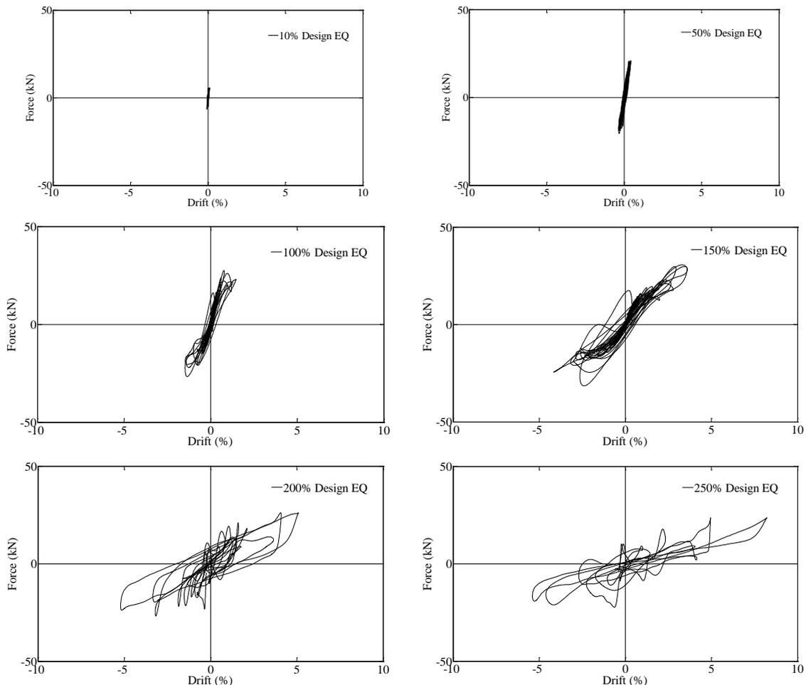
Figure 4. Measured force versus drift ratio at different stages of the test
