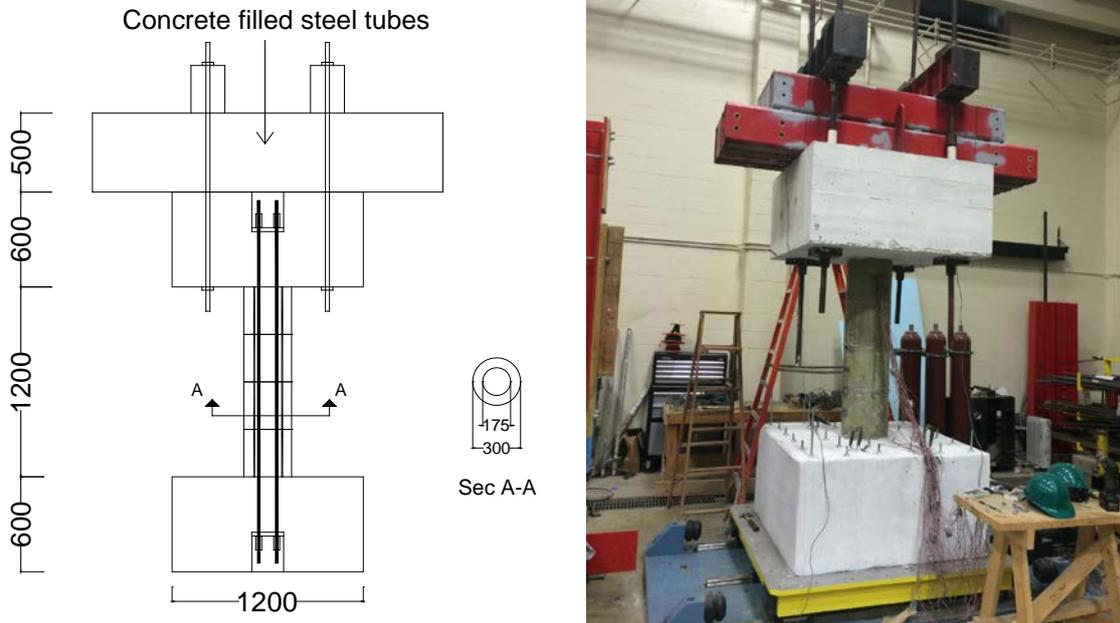
Figure 1. Configuration and dimensions of the test specimen
