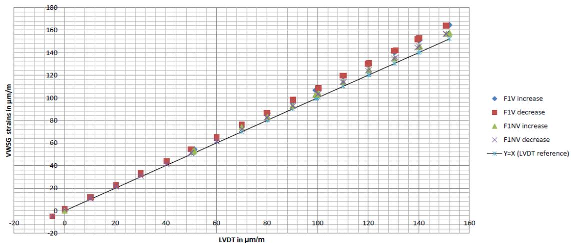
Figure 4: Strain (in  $\mu\text{m}/\text{m}$ ) measured by VWSG versus strain (in  $\mu\text{m}/\text{m}$ ) measured by LVDT. Comparison of the response of a new extensometer (Creep 2 A = F2NV) and an aged extensometer (Creep 2B = F2V) relative to the LVDT reference
