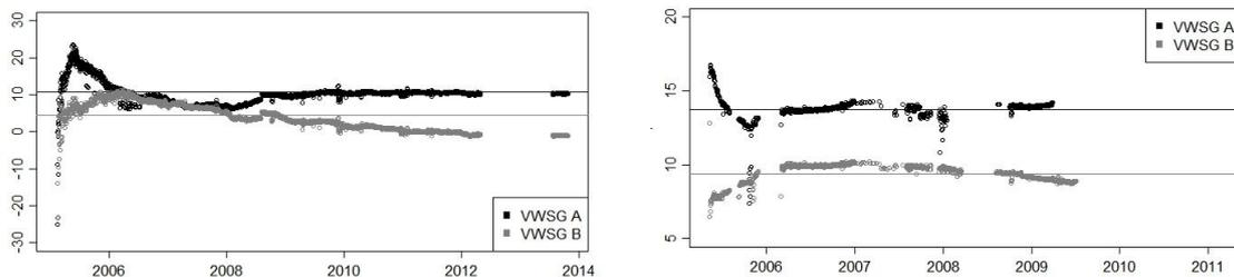
Figure 3: Overestimation (in %) by VWSG over time for shrinkage 3 (left) and creep 2 (right) tests.
