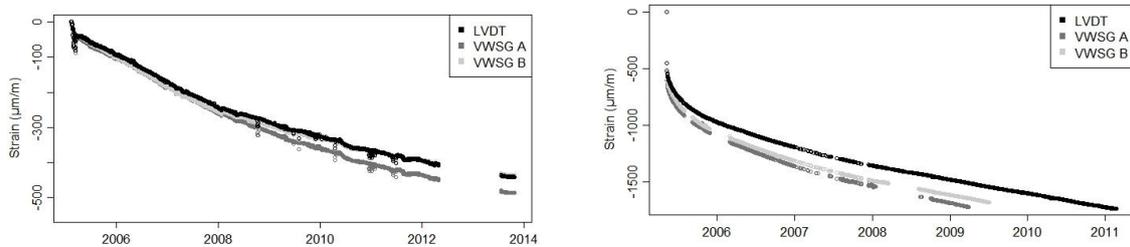
Figure 2: Strain (in  $\mu\text{m/m}$ ) versus time for shrinkage 3 (left) and creep 2 (right) tests.
