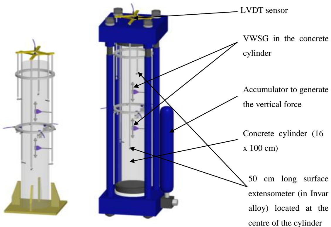
Figure 1: Concrete cylinder for measuring shrinkage (left) and creep (right), with the accumulator to generate the vertical force).
