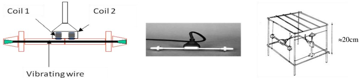
Figure 1: VWSG for the measurement of strain inside concrete.
