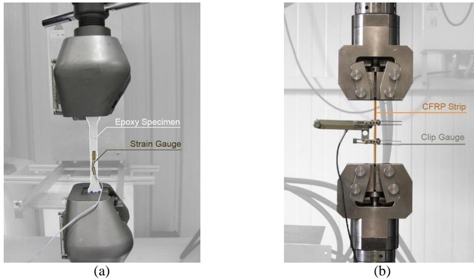
Figure 1. Overview of the test setup of the: (a) epoxy adhesive; (b) CFRP laminate strip.
