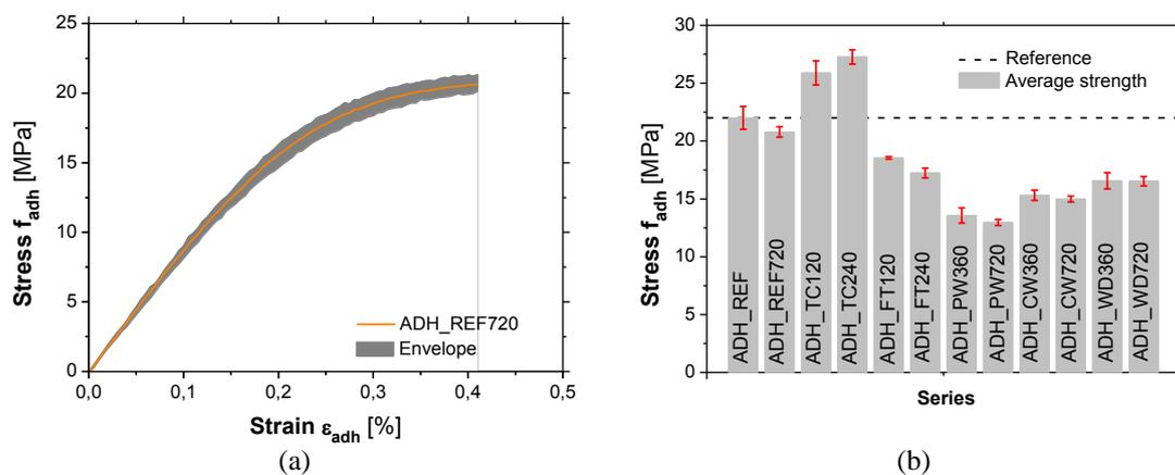
Figure 2. Epoxy adhesive: (a) typical stress-strain curve; (b) Tensile strength obtained in each series.
