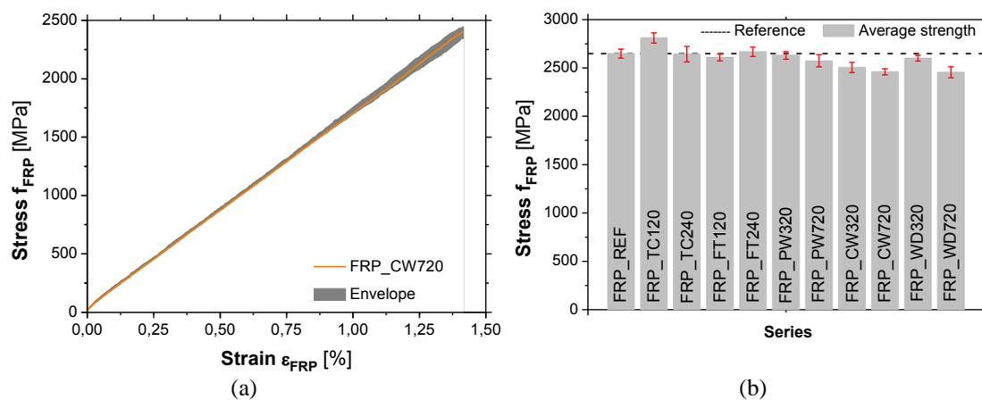
Figure 3. CFRP laminate strip: (a) typical stress-strain curve; (b) Tensile strength obtained in each series.
