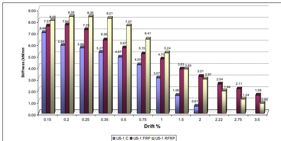
Figure 5. Specimens stiffness value at each drift level.
