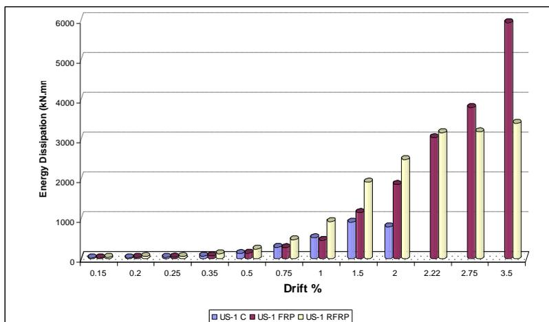
Figure 7. Dissipated energy at each drift level for all specimens.
