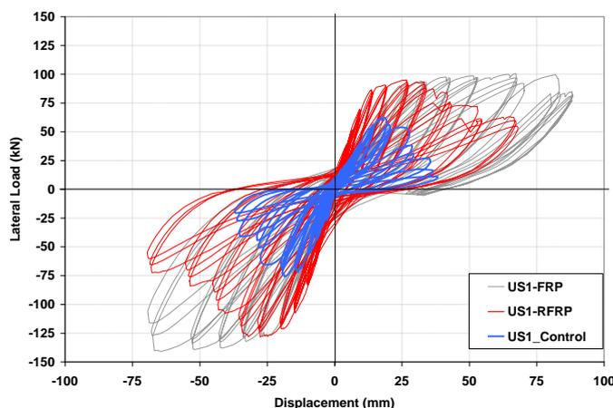
Figure 2. Lateral load versus displacement.
