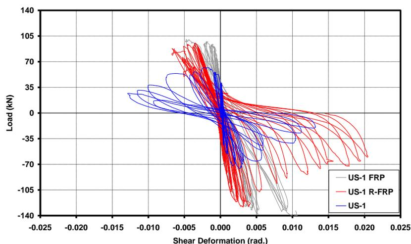
Figure 3. Shear deformation versus lateral load.
