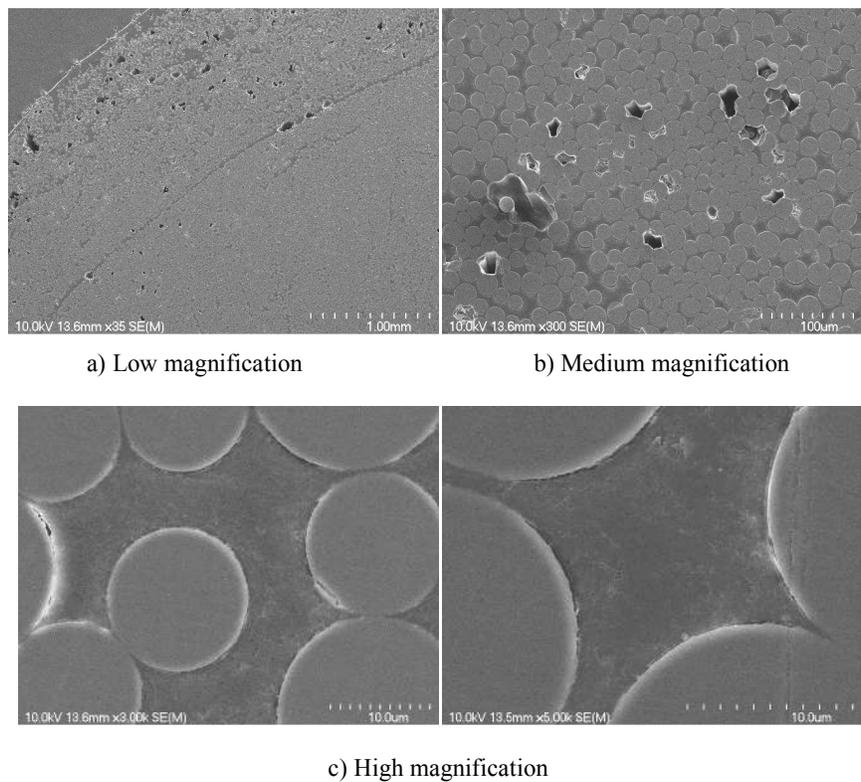
Figure 2. SEM micrographs of the cross-section of the BFRP 16-mm-diameter at different magnifications
