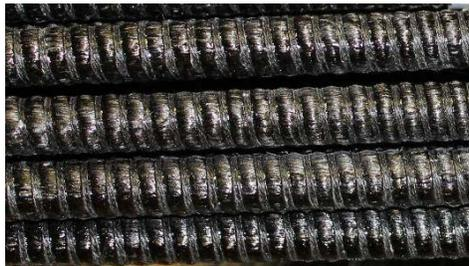
Figure 1. BFRP bars used in this study.
