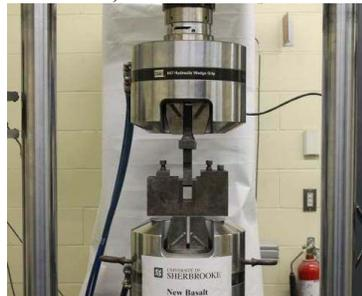
b) Transverse shear test
