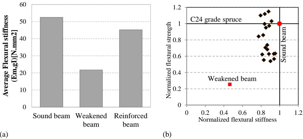
Figure 4. Test results regarding (a) the average flexural stiffness and (b) the flexural strength and stiffness normalized to the sound C24 grade spruce beam.
