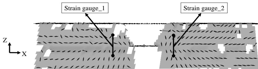
Figure 8. Location of strain gauges and direction of major strain on the bottom surface of the timber beam.
