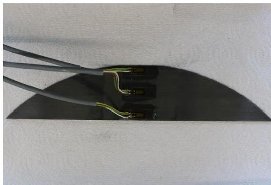
Figure 2. Strain gauges configuration.
