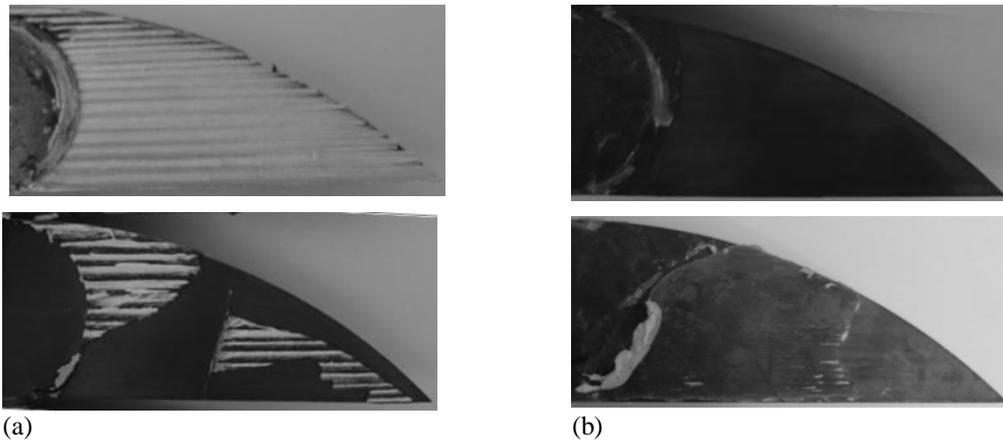
Figure 6. Failure in the (a) timber fibers and (b) interface between the timber and adhesive.
