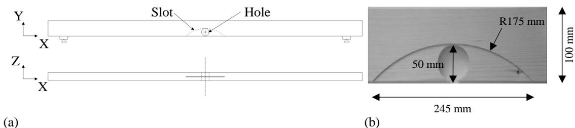
Figure 1. (a) Position of knot and slot at the mid-length of the beam and (b) size and shape of slot for inserting reinforcement strip.
