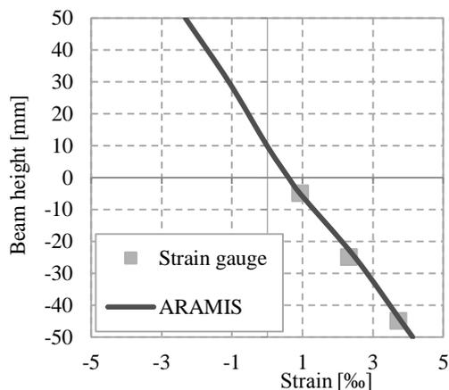
Figure 7. Distribution of horizontal strain through height of the beam.
