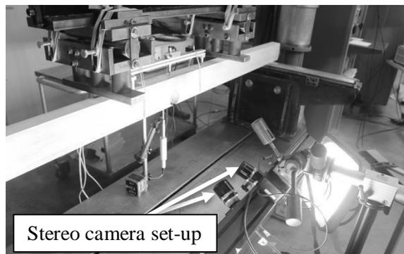
Figure 3. 3D image correlation system installation.
