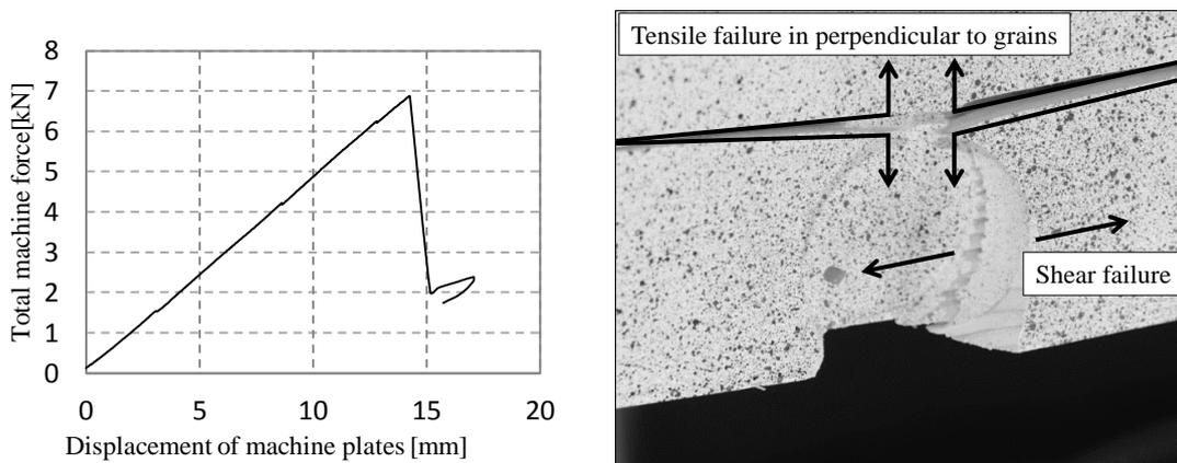
Figure 5. (a) Load-deflection diagram of a locally reinforced beam and (b) the pronounced failures resulting the drop.
