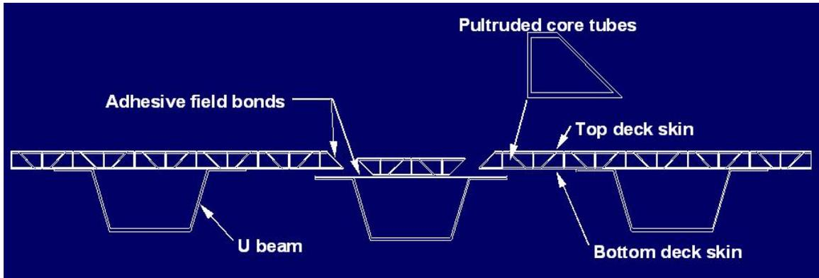
Figure 3. Typical Trapezoidal-Shape Cross-Section.
