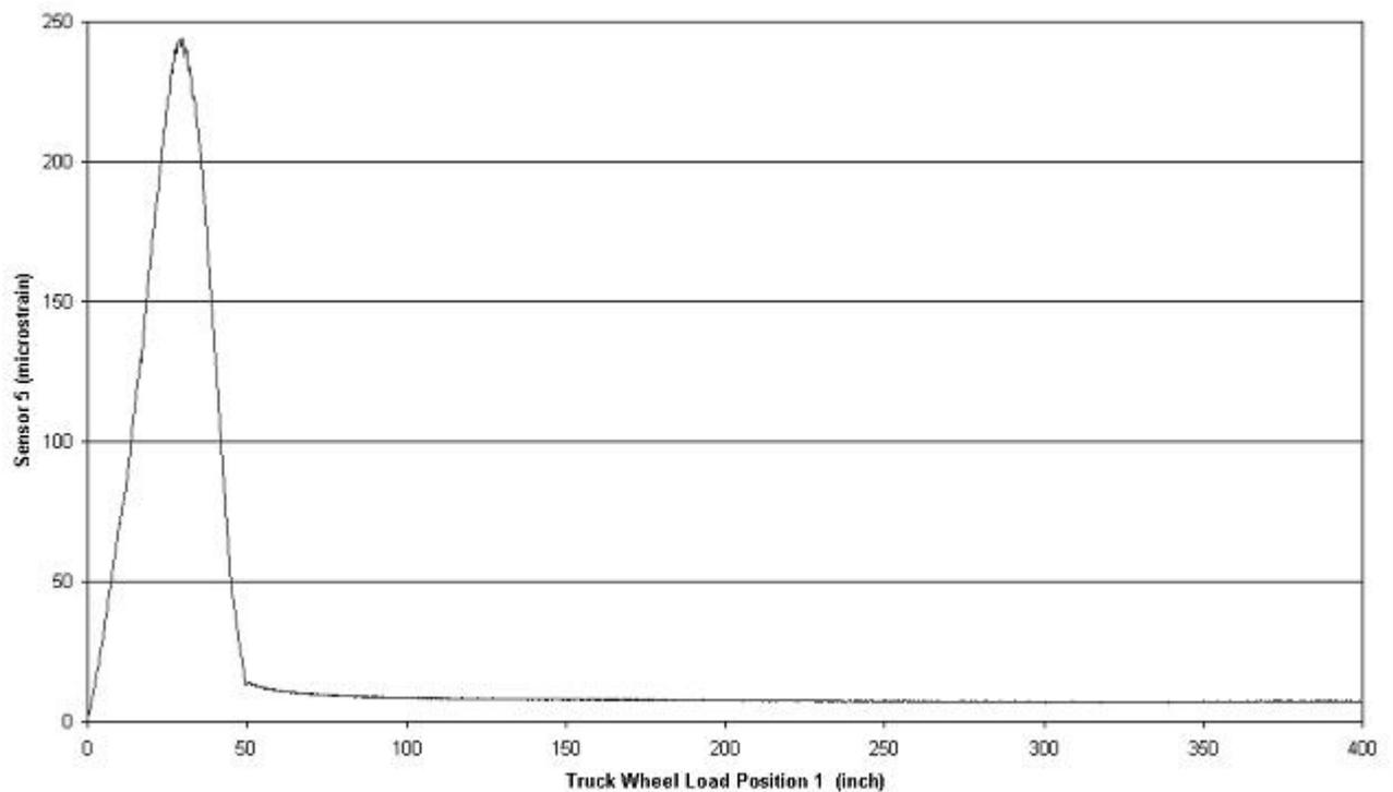
Figure 4. Bridge Response Due to Truck Load Test at Crawling Speed.
