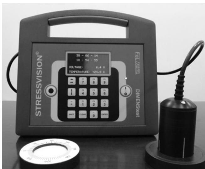
Fig. 2 Indicator of Mechanical Stresses (IMS), probe (transducer) and 2 calibration rings.
