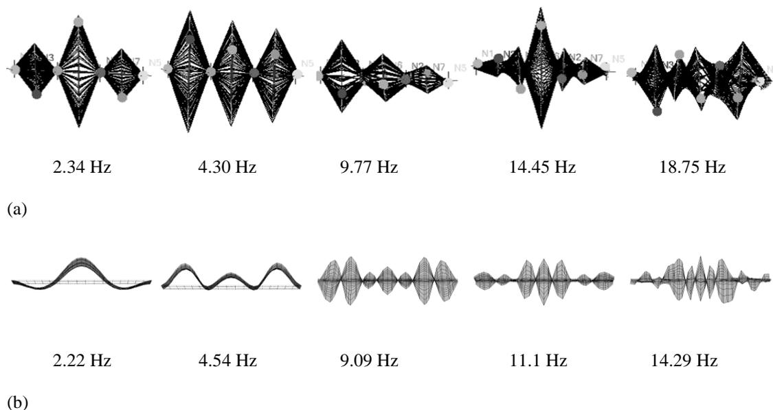
Figure 3. Comparison of analysis results (a) results of measurement (b) results of FEM.
