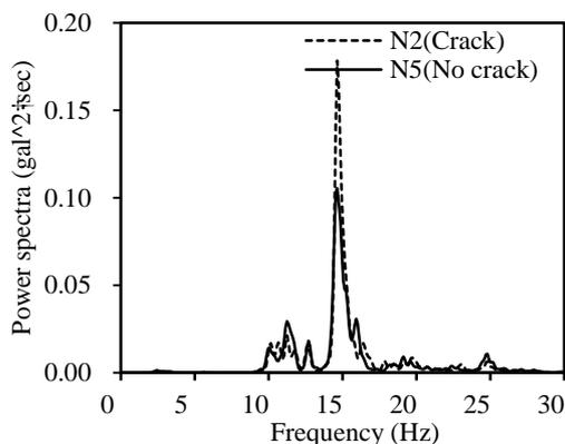
Figure 4. Power spectra when a vehicle is crossing.
