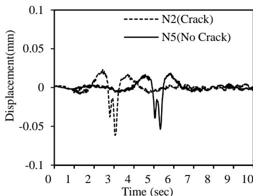
Figure 5. Displacement when a vehicle is crossing.
