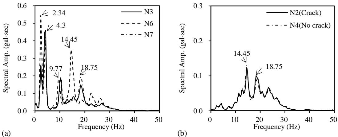
Figure 2. Fourier spectral (a) center of spans (b) intermediate supporting points.
