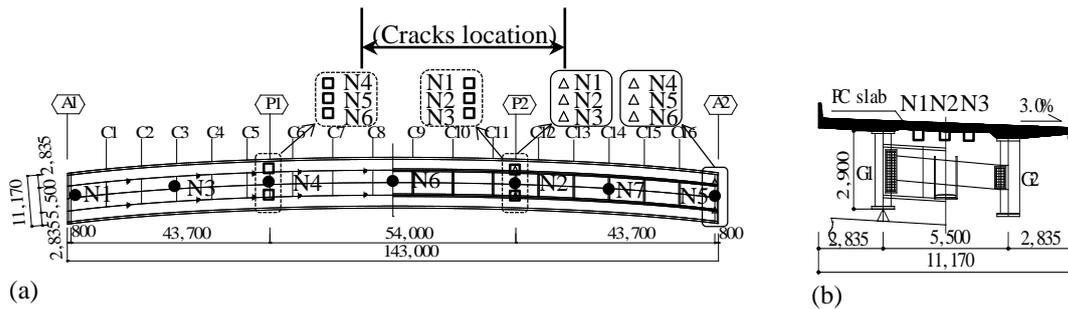
Figure 1. Bridge drawing and sensor setting cases (a) plan of the bridge (b) cross section of P2 (Case 1: ●, Case 2: □, Case 3: △).
