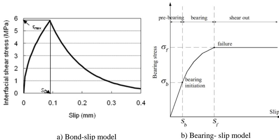
Figure 1. Interfacial stress-slip relationship adopted for (a) the EB FRP strengthened specimens and (b) the mechanically fastened FRP strengthened specimens.
