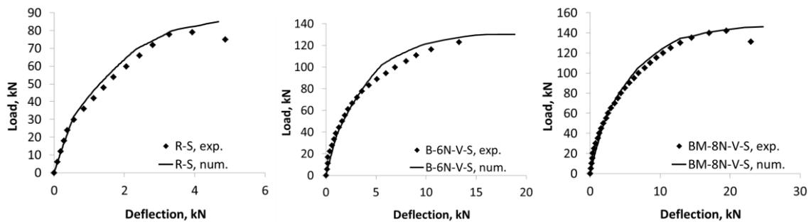
Figure 3. load deflection comparison for a reference specimen, EB and hybrid EB/MF specimen.
