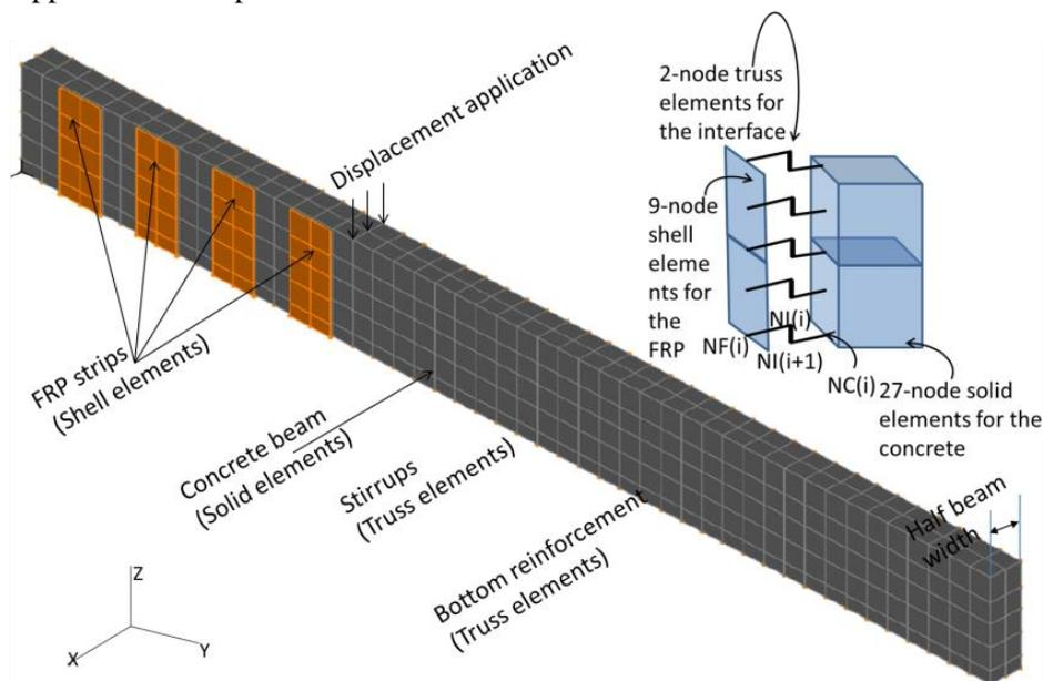
Figure 2. Finite element model for a strengthened specimen.
