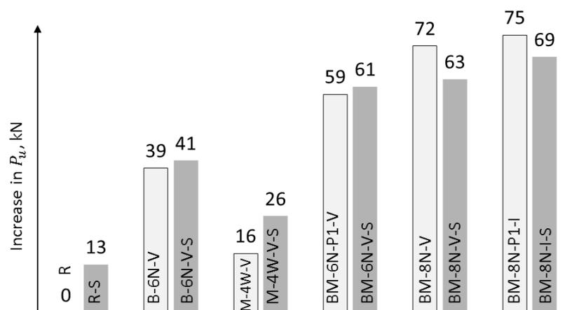
Figure 5. Load increases for specimens with and without transverse steel reinforcement, kN.
