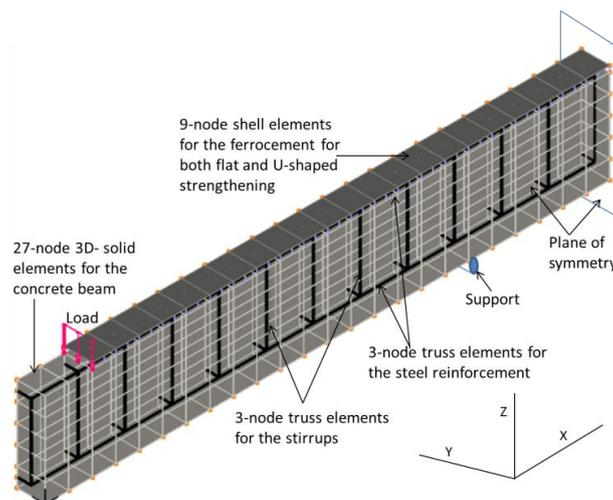
Figure 2. Finite element model for a flat-shaped strengthened specimen.
