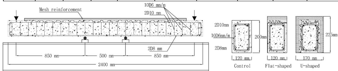
Figure 1. Beam characteristics and dimensions.
