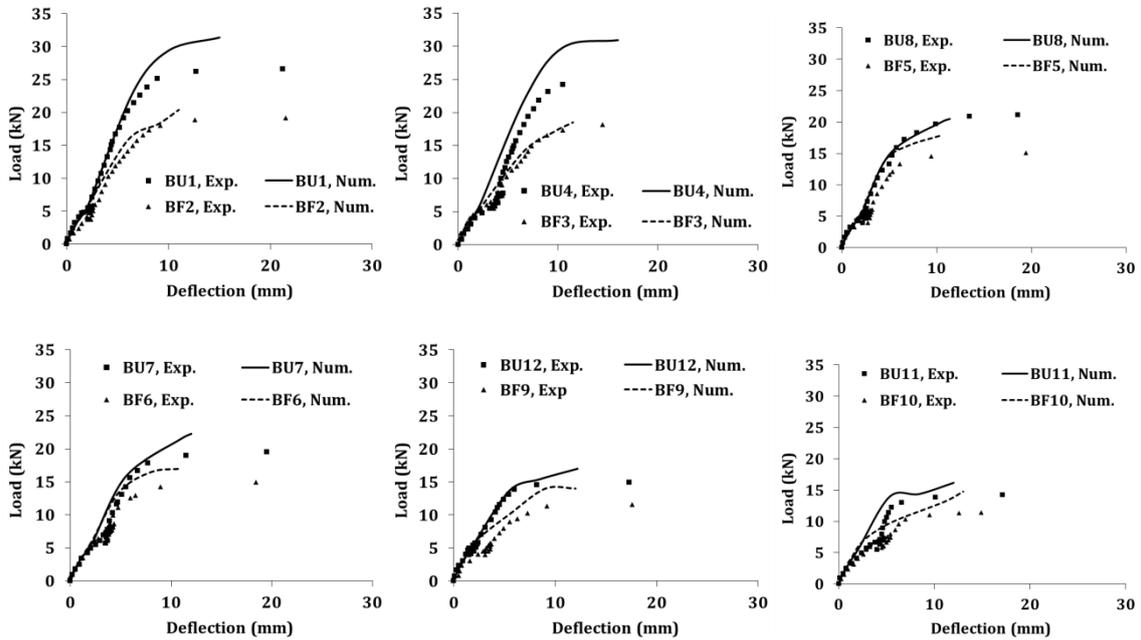
Figure 3. Numerical versus experimental load-deflection relationships for the entire specimens.
