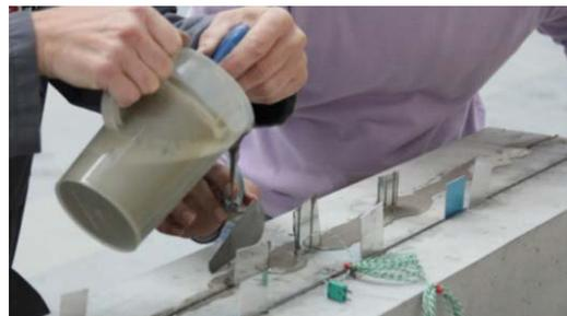
Figure 3: Embedding Fe-SMA strips with cement based grout.
