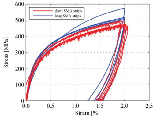
Figure 6: Prestraining of short and long strips.
