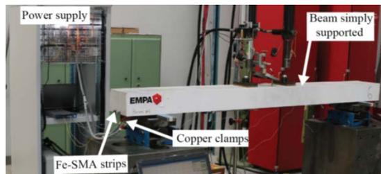
Figure 4: Beam No. 6 equipped for activation.
