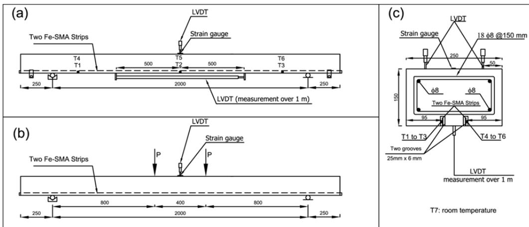
Figure 1: Drawing of Fe-SMA strengthened beams; a) setup for activation, b) setup for loading, and c) cross section of beams. T1 to T7 are thermocouple, all dimensions are in mm.
