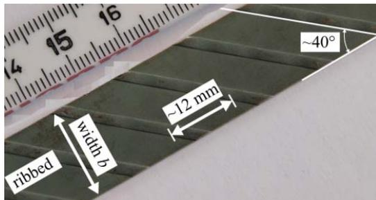
Figure 2: Detailed view of ribbed Fe-SMA strips.
