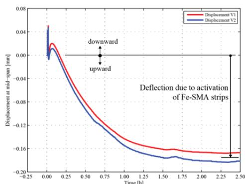
Figure 8: Behavior of Beam No. 6 during and after activation.
