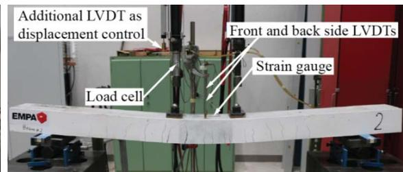
Figure 5: Beam No. 2 in loading setup after failure.
