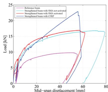
Figure 9: Load -mid-span displacement diagrams of the examined beams up to failure.
