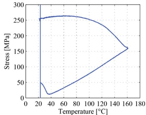
Figure 7: A typical recovery stress diagram of Fe-SMA strip specimen.
