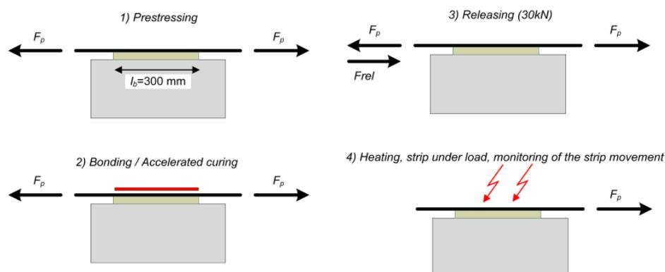
Figure 4. Anchoring and heating procedure for the temperature stability tests for prestressed CFRP strips.
