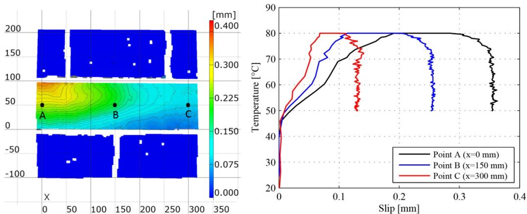
Figure 8. Measurements during the simulation of the asphalt scenario for test No.3: (Left) Longitudinal displacements at the beginning of the cooling down (80 °C); (Right) Relative strip displacements at three different points.
