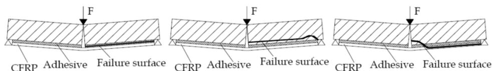
Figure 2. Failure modes observed for different temperature values (Di Tommaso et al. (2001)): (Left) Adhesive failure; (Middle) Concrete failure; (Right) Failure due to CFRP delamination.
