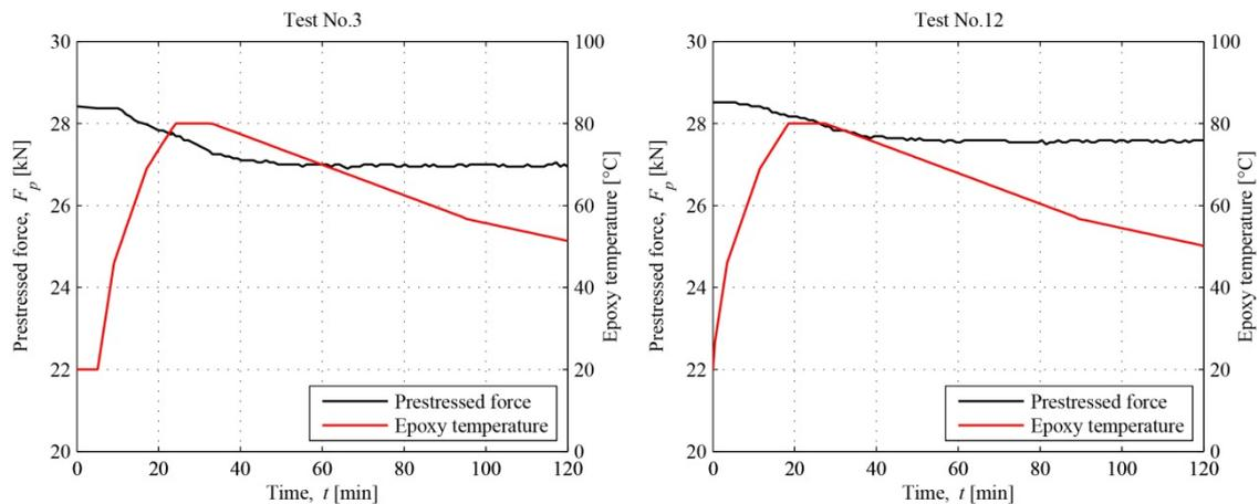
Figure 7. Evolution in time of the prestress force during the simulation of the asphalt scenario: (Left) Test No.3; (Right) Test No.12.
