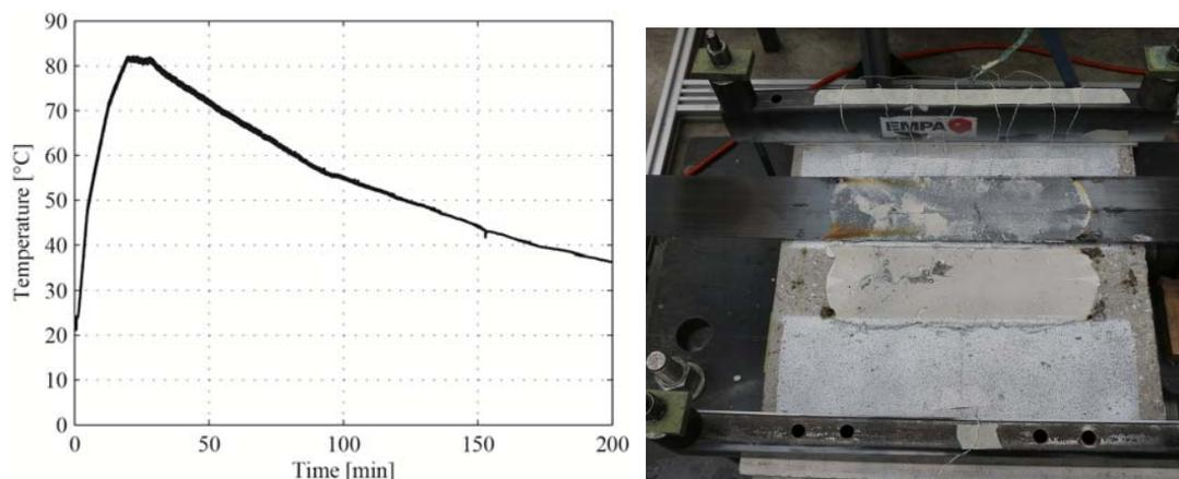
Figure 6. (Left) Epoxy temperature measured during the simulation of the asphalt scenario; (Right) Test No.12 after failure at a constant temperature of 80°C.
