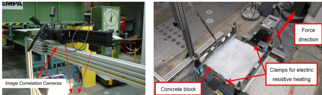
Figure 5. Setup for the temperature stability tests for prestressed CFRP strips.
