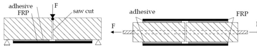
Figure 1. Typical test set-up in small scale specimens (Klamer et al. (2008)): (Left) Three point bending test; (Right) Double-lap shear test.
