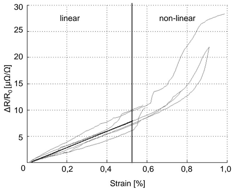
Figure 5. Strain-Resistance Diagram of Carbon Roving 2
