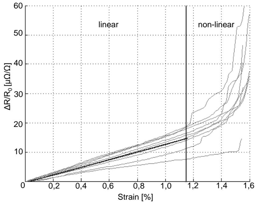
Figure 4. Strain-Resistance Diagram of Carbon Roving 1
