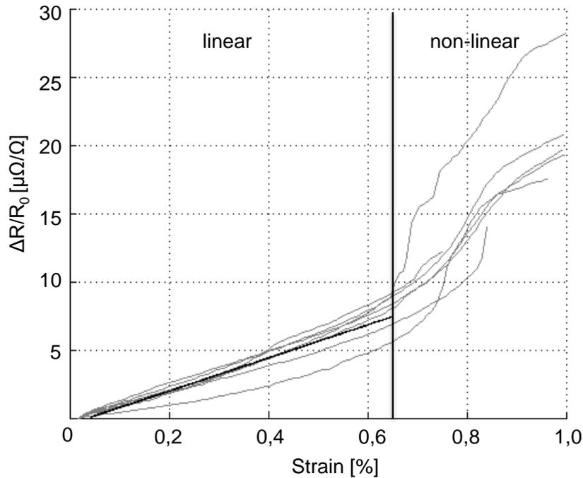
Figure 6. Strain-Resistance Diagram of Carbon Roving 3
