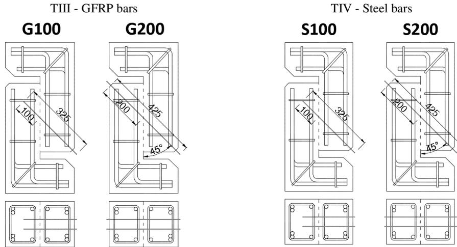
Figure 5. Specimen details
