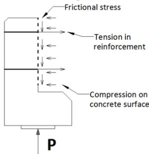
Figure 6. Shear-friction model
