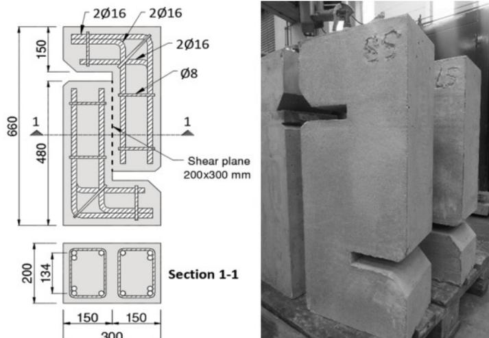
Figure 1. Steel reinforcement of the specimens and their appearance after casting
