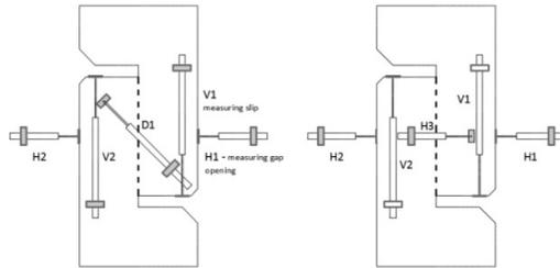
Figure 3. Positions of LVDTs
