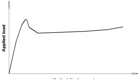
Figure 7. Typical load/vertical displacement diagram for specimens reinforced with FRP bars
