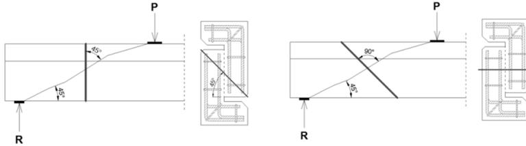
Figure 4. Different angles of bar insertion
