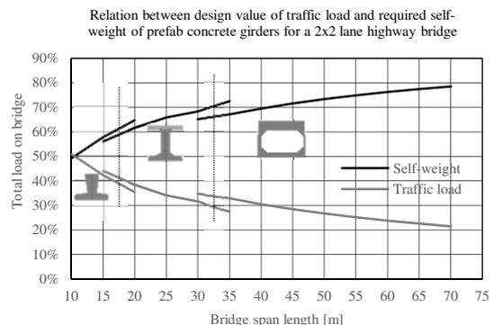
Figure 10. Traffic load vs. self-weight percentage
