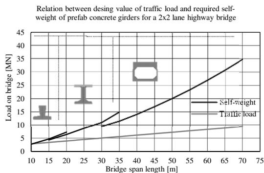
Figure 9. Traffic load vs. self-weight absolute
