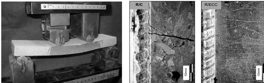
Figure 8. SHCC in four point bending test, crack pattern in ordinary concrete and in SHCC (Li, 2007).
