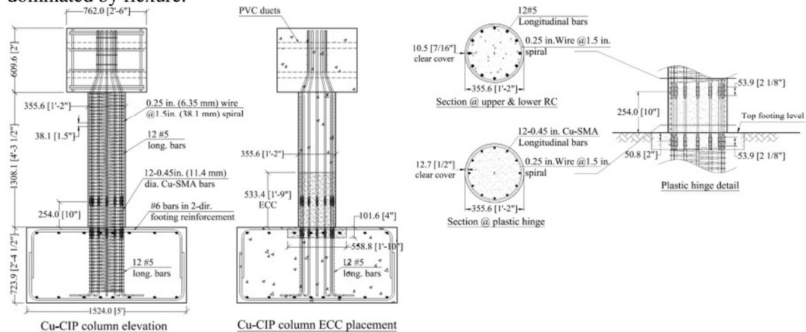
Figure 1. Quarter-scale column model dimensions and details.
