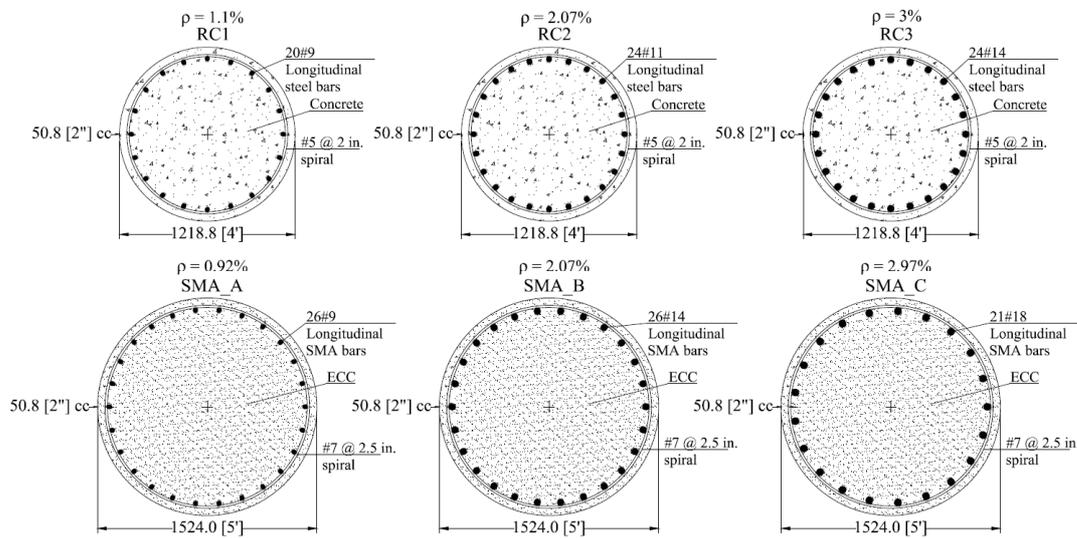
Figure 5. RC and ECC/SMA column sections.
