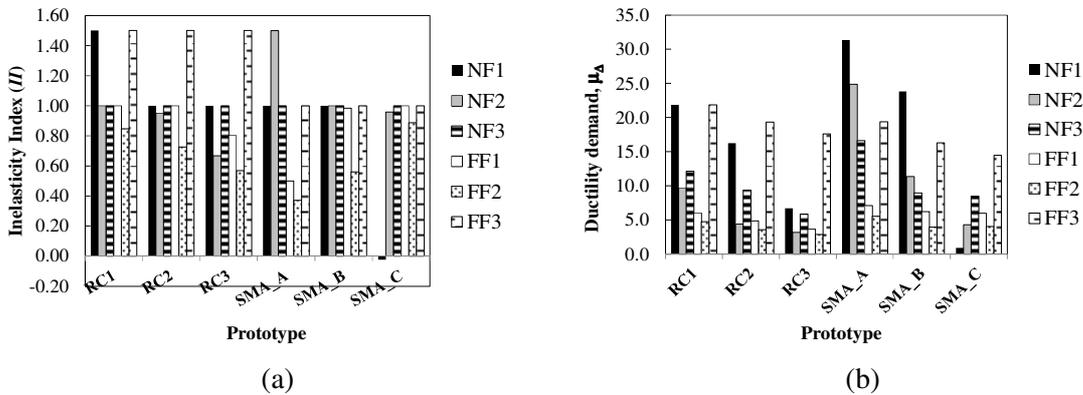
Figure 6. Calculated inelasticity index and ductility demand for all columns.
