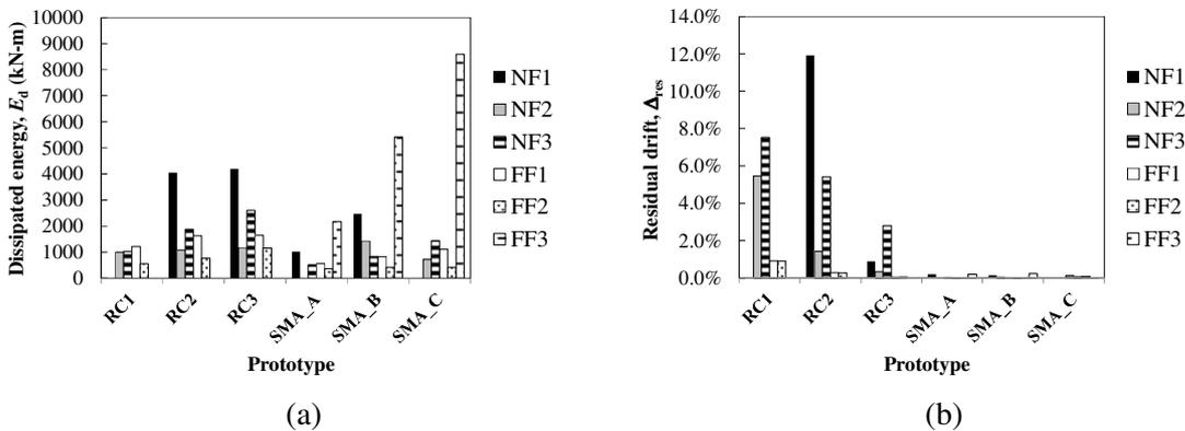
Figure 7. Calculated dissipated energy and residual drift for all columns.
