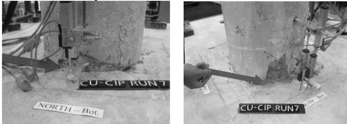
Figure 4. Plastic hinge damage after 12% drift. Left: north side, right: south side.
