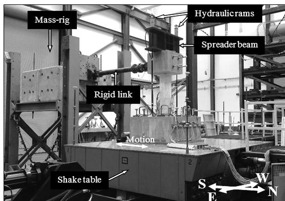
Figure 3. Shake table test setup.
