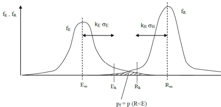
Figure 1: Probabilities of the action E and resistance R
