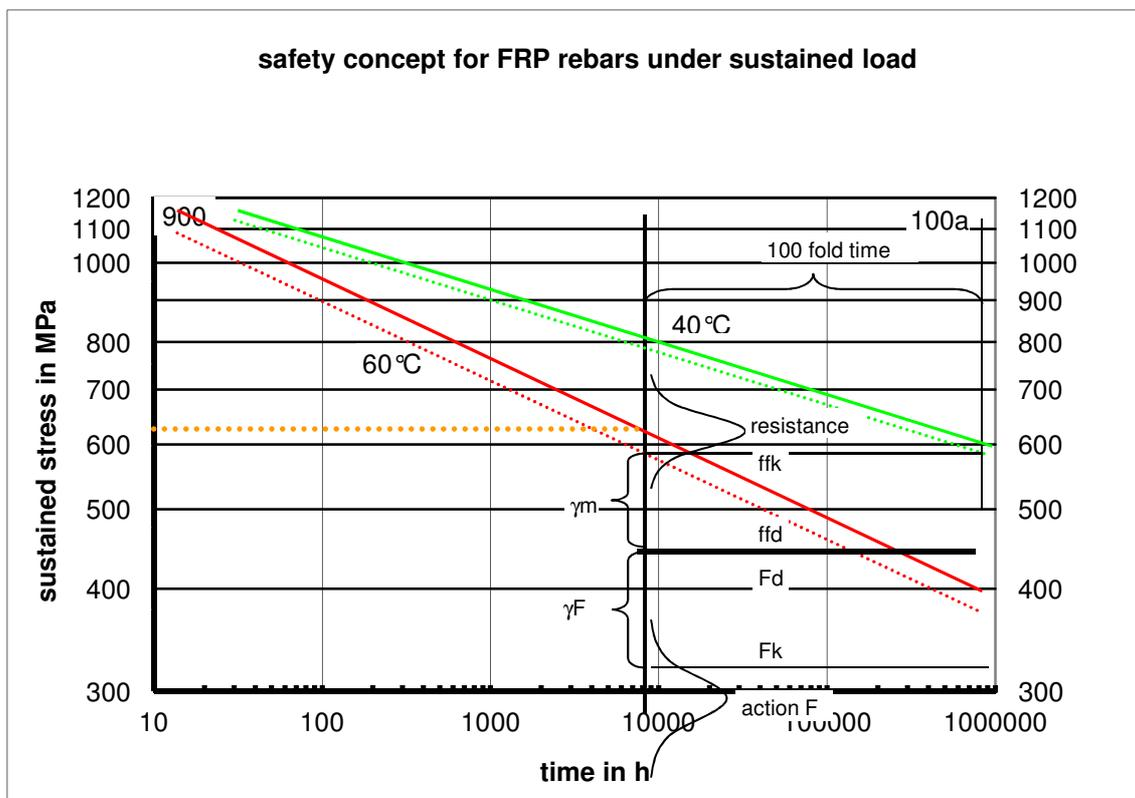
Figure 2: Safety relations for time dependent FRP rebars under load
