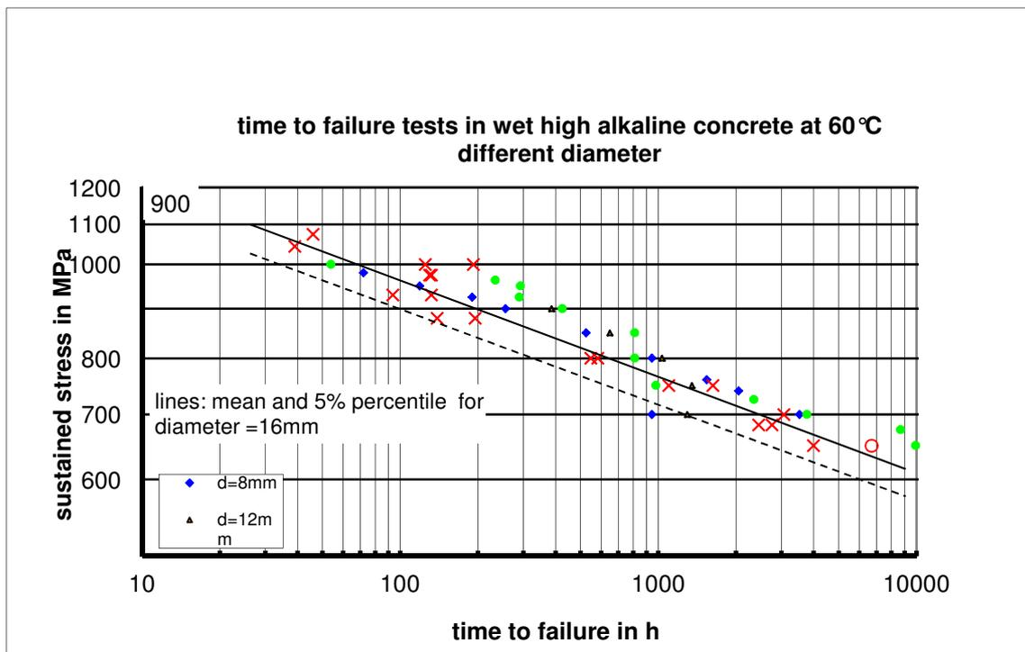
Figure 4: Creep rupture tests with different diameters
