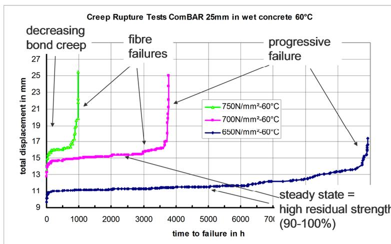
Figure 3: Creep with different incidents
