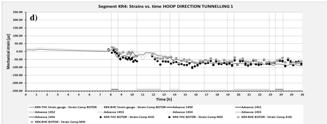
Figure 3. Strain history of segment KR4 centre for the first 26h after ring erection: a) Actual longitudinal strains (VWSG) and cylinder thrust; b) Mechanical longitudinal strains (VWSG) and cylinder thrust; c) Actual and mechanical hoop strains and temperature from VWSG; d) Mechanical hoop strains (BOTDR and VWSG).
