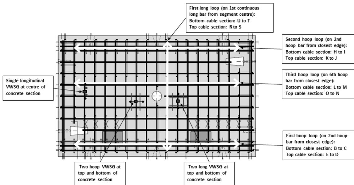
Figure 2. Instrumentation topology and location of box-outs in a precast concrete segment.
