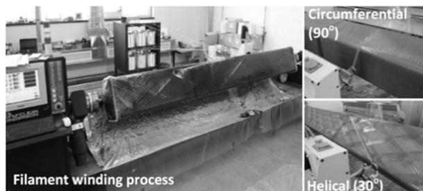
Figure 1. Filament winding process
