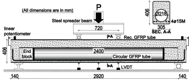
Figure 3. Schematic of test setup
