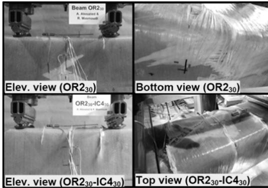
Figure 4. Failure pattern of CFFT beams
