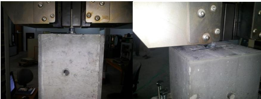
Figure.6 Specimen1 under uniaxial tension force
