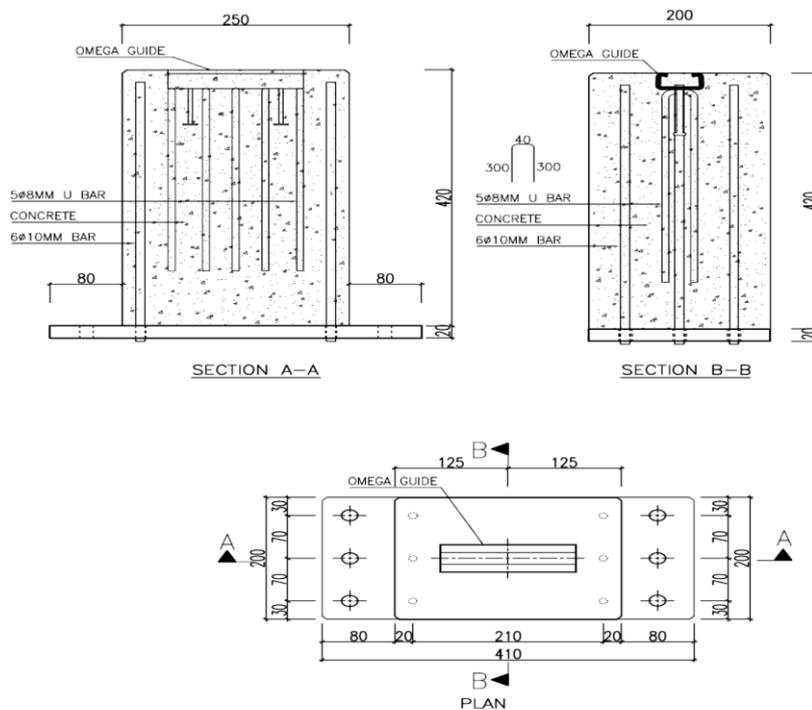
Figure 5: Specimen with reinforcement bars welded to the channel
