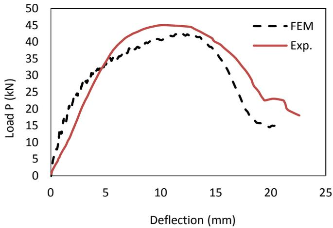
Figure.9 load- deflection curve of the experimental work and finite element analysis
