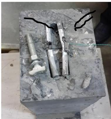
a) Experimental damage and slip of channel related to concrete
