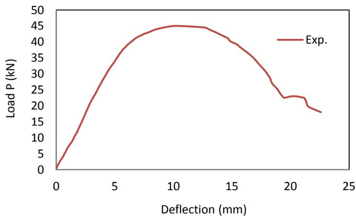
Figure.7 Load- deflection curve of SP1
