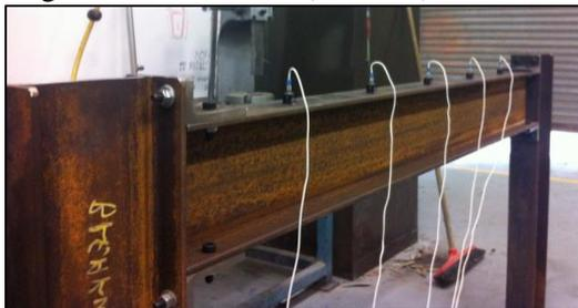
Figure 3. Steel Frame Structure Photograph (far-end accelerometer data used only) (Ay et al., 2013)
