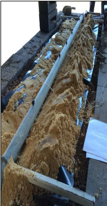
Figure 6. Steel pipe test structure photograph (damage scenario 3 shown)
