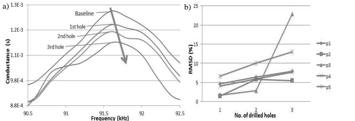
Figure 3. Signal processing (a) Conductance signals of surface PZT 5 (b) Conductance RMSD of surface PZTs – damages by drilling holes
