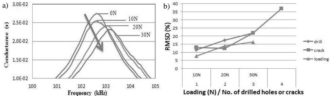
Figure 5. Signal processing (a) Conductance signals of magnetic PZT (b) Conductance RMSD of magnetic PZT – damages by drilling holes, crack and load test
