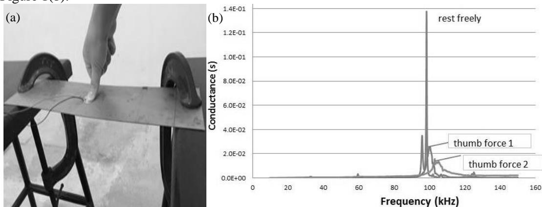
Figure 1. (a) Photo and (b) conductance signals of thumb force bonded PZT
