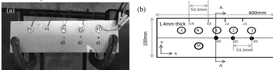
Figure 2. (a) Photo and (b) schematics of specimen with details of 5 surface PZTs and 1 magnetic PZT
