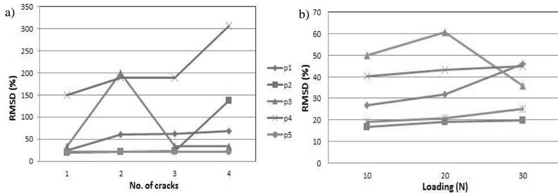
Figure 4. Conductance RMSD for surface PZT – (a) crack test, (b) load test
