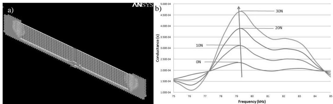
Figure 6. Load test – (a) Numerical screenshot of the model (b) Numerical conductance signals
