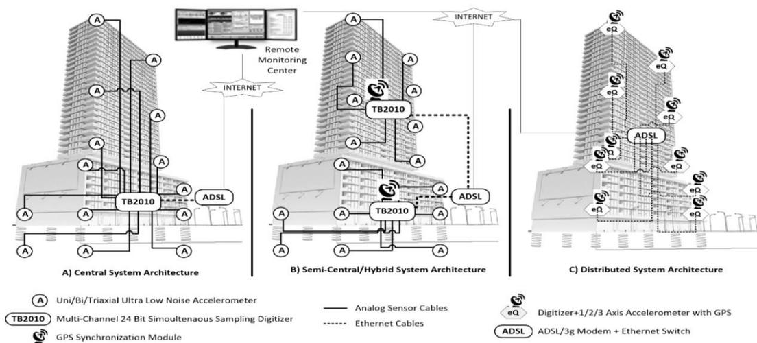
Figure 6. Three different architectures for installing instruments and sensors on buildings.
