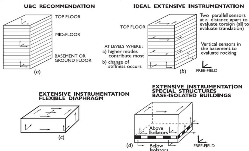
Figure 3. Sensor locations on buildings, taken from the report for which Çelebi(2002) prepared for USGS.
