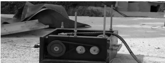
Figure 2. TESTBOX<sup>TM</sup>-SHAKER Eccentric Mass Shaker in “Earthquake Performance Tests on Full Scale Existing Buildings” project conducted by Istanbul Technical University Civil Engineering Department.
