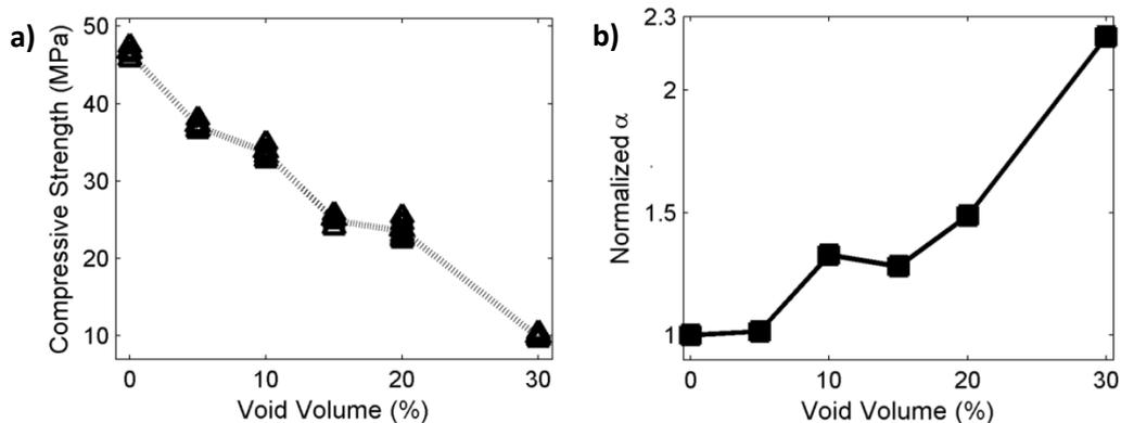
Figure 5. (a) Compressive strength of the beam sections (b) the attenuation coefficient
