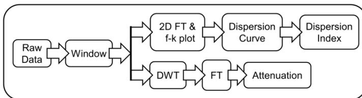
Figure 4. Signal processing algorithm.
