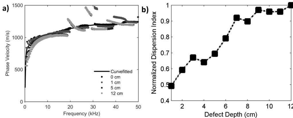
Figure 3. (a) Dispersion curves for case D00, D01, D05, D12 (b) Dispersion index vs. damage case.
