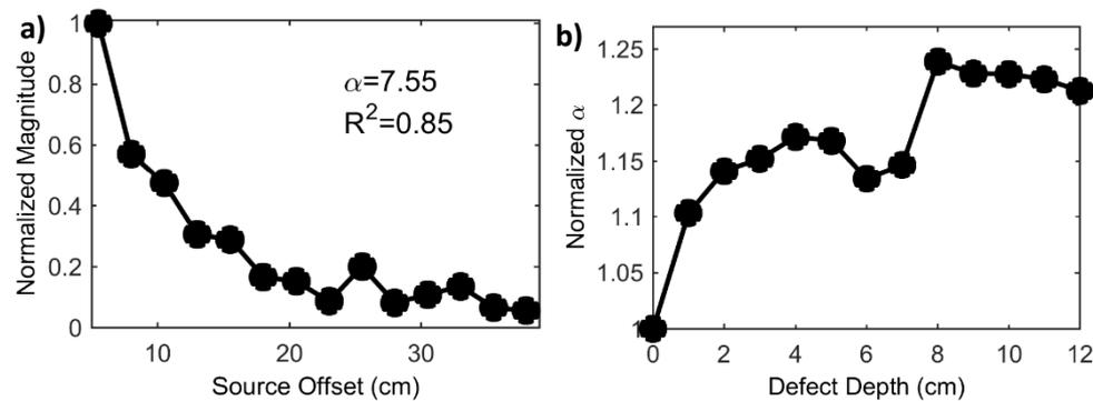
Figure 2. (a) Attenuation trends (case D00), (b) the  $\alpha$  computed for each damage case.
