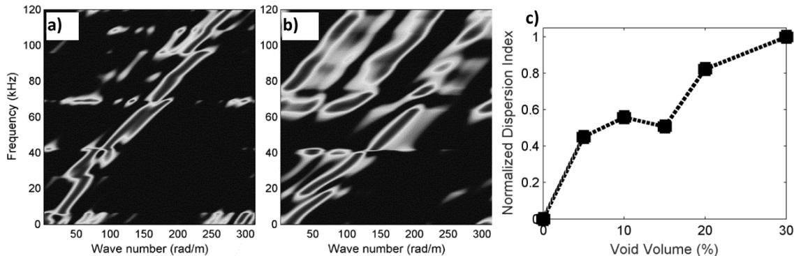
Figure 7. The f-k plot for (a) B00 and (b) B30, (c) the dispersion index vs. void volume.
