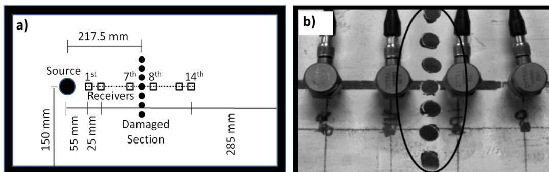
Figure 1. (a) Testing configuration (Not to scale) (b) the damaged section on the rig.
