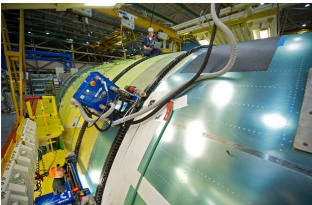
Figure 7. Application of the Flex Track system on the fuselage of an airplane equipped with a drilling machine, Thompson et al. (2005), courtesy of Boeing.
