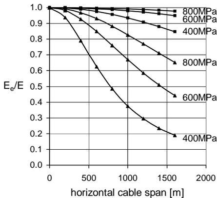
Figure 9. Relative equivalent modulus of elasticity  $E_e/E$  versus the horizontal cable span for CFRP and steel cables according to Eq. 1. The applied cable stress is given as a parameter. The constants are:  $E_{\text{steel}}=210$  GPa;  $E_{\text{CFRP}}=165$  GPa;  $\rho_{\text{steel}}=7.8\text{t/m}^3$ ;  $\rho_{\text{CFRP}}=1.6\text{t/m}^3$ . The three curves at the top end (■) represent CFRP stays and those three at the bottom end (▲) steel stays.
