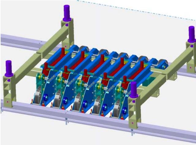
Figure 6. Automated device for simultaneous application of five pre-tensioned CFRP strips; Meier (2012/1).
