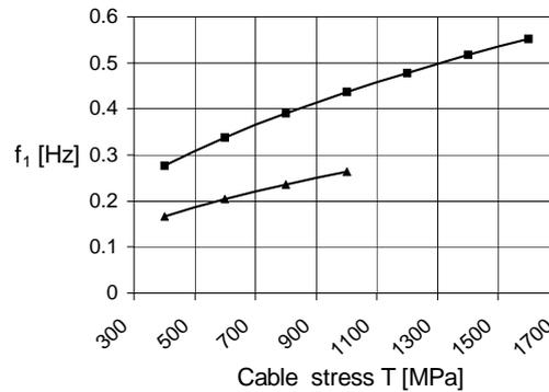
Figure 11. Frequencies  $f_1$  vs. cable tension  $T$  for cables of 650 m length. The curve at the top ( $\blacksquare$ ) represents a CFRP stay and that at the bottom ( $\blacktriangle$ ) a steel stays. Cable mass per meter: CFRP 21 kg/m, Steel 102 kg/m. Assumption:  $EI \rightarrow 0$  according to Girmscheid (1987).
