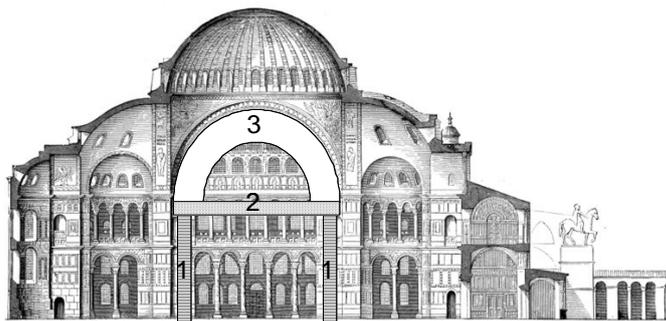
Figure 8. Cross section of Hagia Sophia: Example for the seismic protection of an arch. 1 = telescopic CFRP columns; 2 = linear CFRP U-profile, open to the top; 3 = deployed tubular earthquake airbag.
