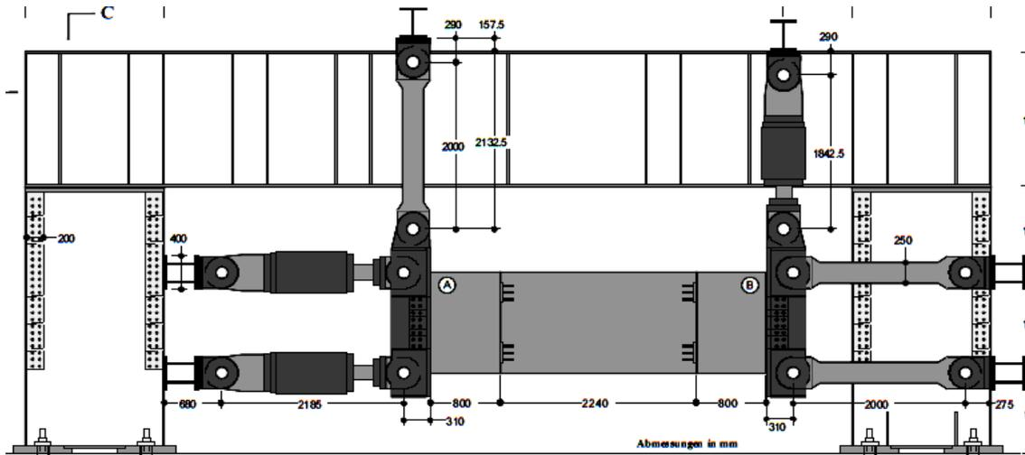
Figure 4. "Beam-Element-Tester" developed by Professor Peter Marti at ETH Zurich.
