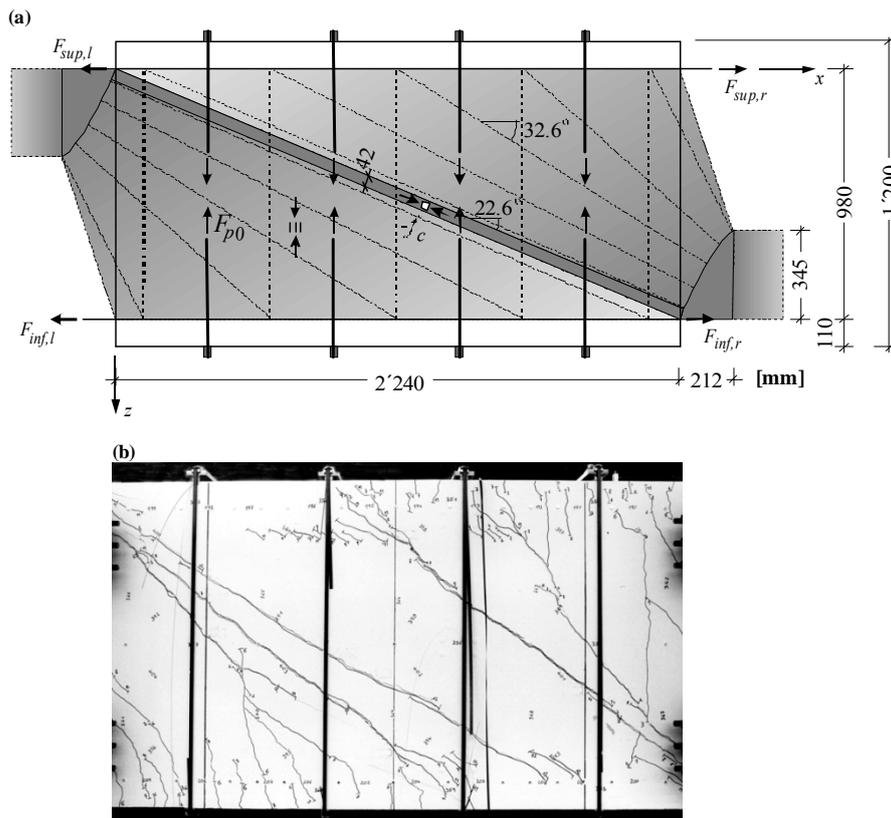
Figure 5. Shear wall ST1 loaded up to  $-635$  kN: (a) on top: discontinuous stress field; (b) on bottom: crack distribution.
