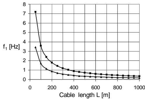
Figure 10. Frequency  $f_1$  vs. cable length. The curve at the top ( $\blacksquare$ ) represents CFRP stays with a cable tension of 1600 MPa and that at the bottom ( $\blacktriangle$ ) steel stays with a cable tension of 1000 MPa. Cable mass per meter: CFRP 21 kg/m, Steel 102 kg/m.
