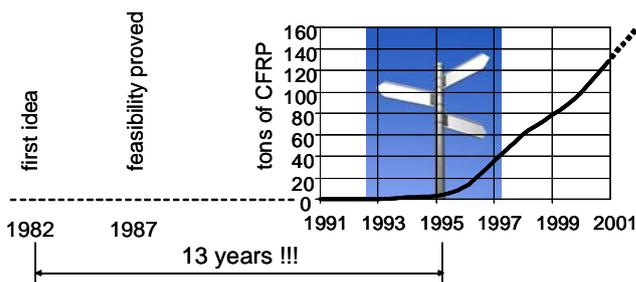
Figure 12. Historic development of the post-strengthening technique with CFRP strips: 1982 first idea, 1987 feasibility proved, 1991 application of the first 6 kg and 1995 commercial take-off. The ascending curve displays the tons of CFRP used per annum in Switzerland.
