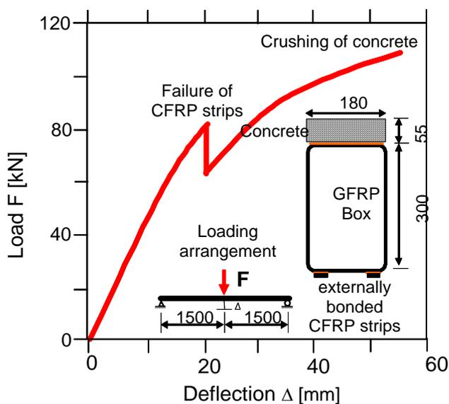
Figure 1. Short time loading test of hybrid GFRP/CFRP/concrete beam; all measurements in [mm].
