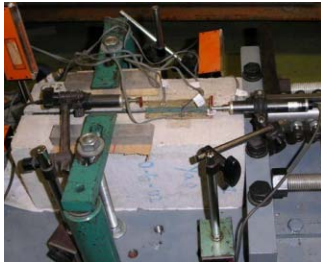
Fig. 4. Setup of single-lap Shear test
