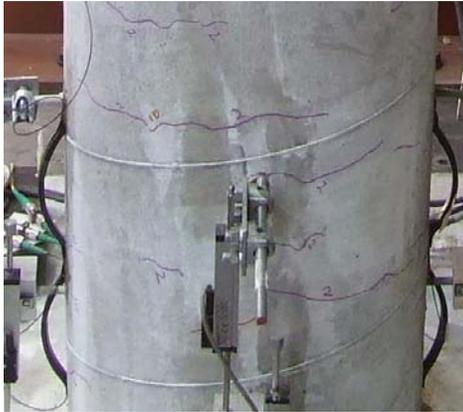
Figure 4 FBG crack sensors on the bridge piers (Bassam, et al, 2011).
