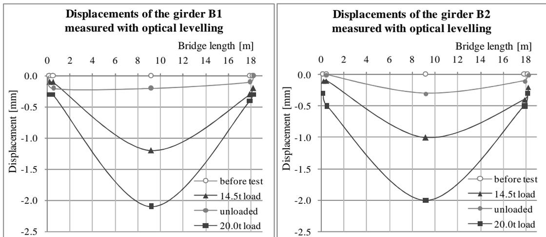
Figure 5. Vertical displacements of the girders at different phases of the test.
