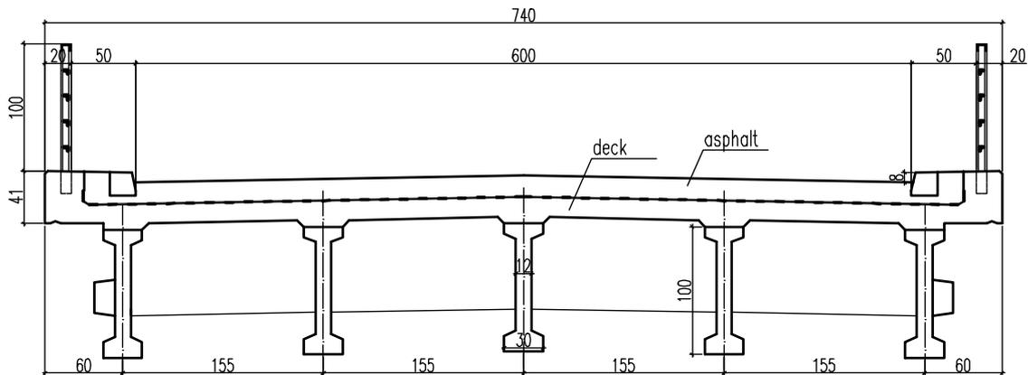
Figure 1. Bridge cross-section.
