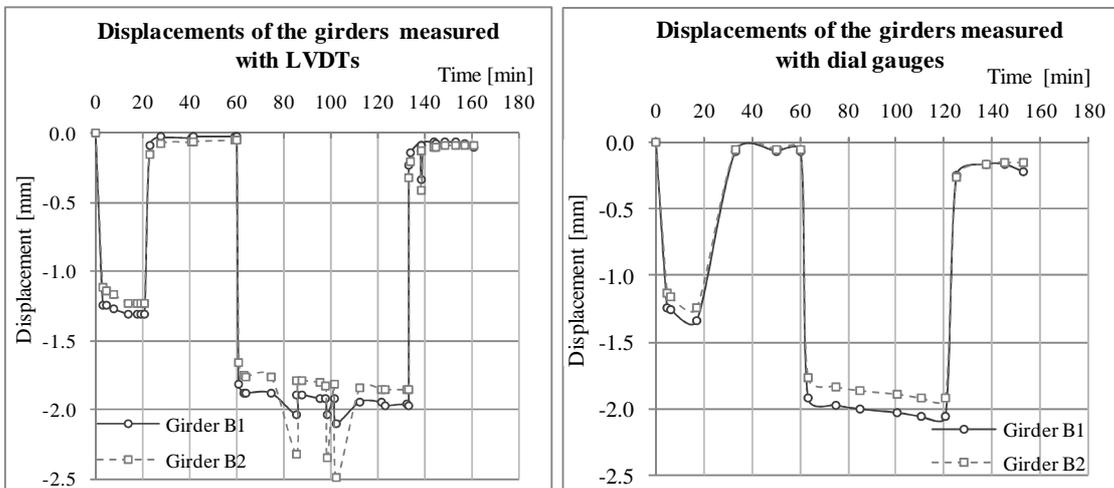
Figure 3. Vertical displacements of the girders' midspan.
