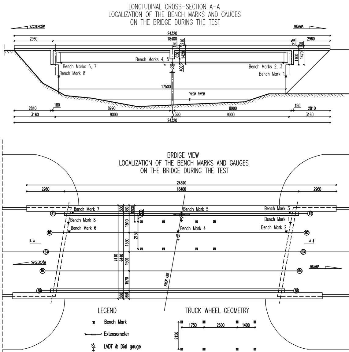
Figure 2. Location of the measuring instruments and the truck on the bridge during the test.
