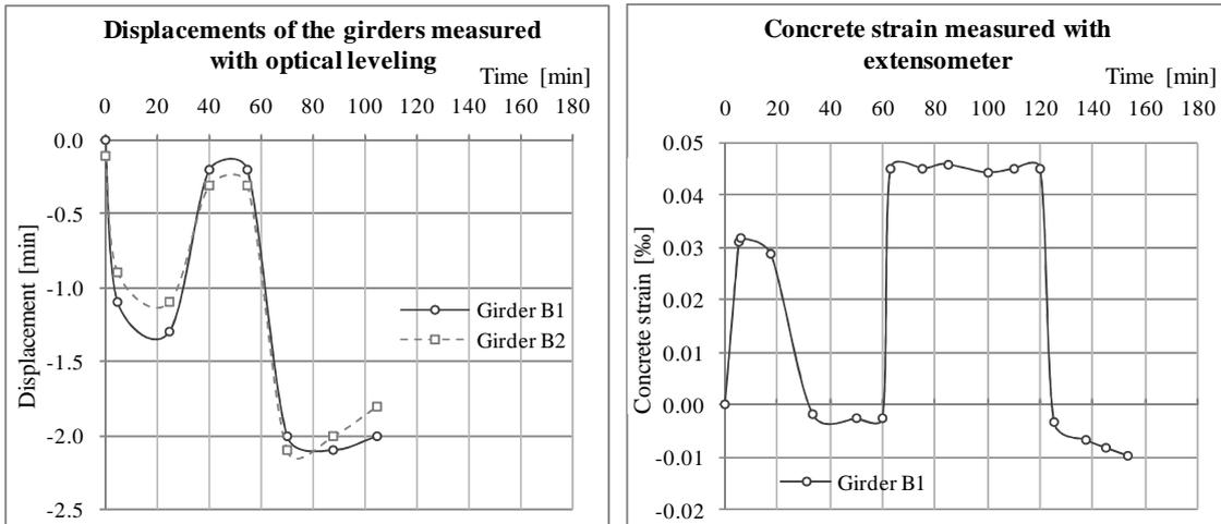
Figure 4. Vertical displacements and concrete strains at the girders' midspan.
