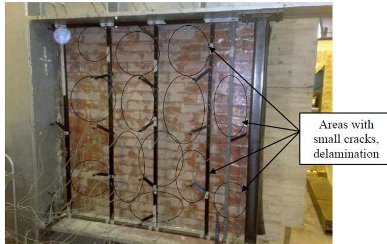
Photo 3. Damage of the wall 2
