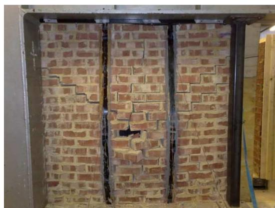
Photo 4. Damage of the Wall 3
