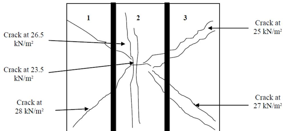
Figure 1. A scheme of the cracks before the collapse, Wall 3
