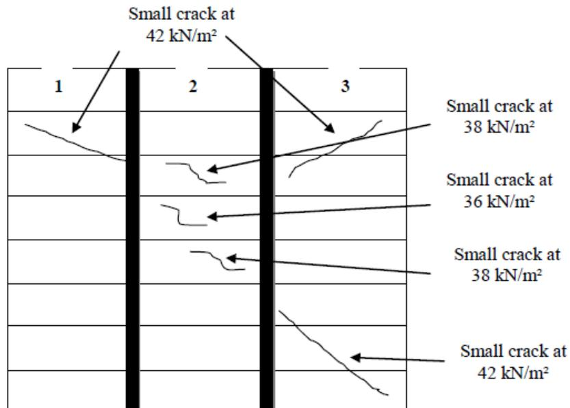
Figure 3. A scheme of the cracks before collapse of wall 5
