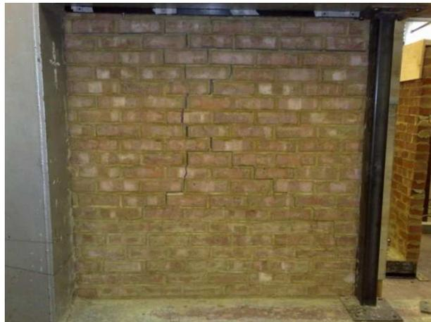
Photo 2. Damage of the control wall (wall 1)
