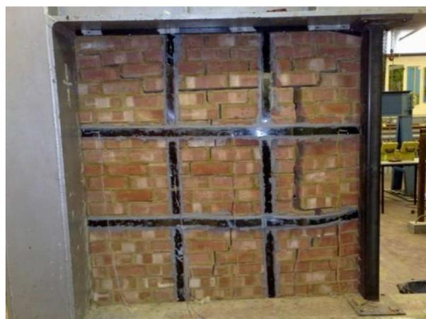
Photo 5. Damage of the wall 4
