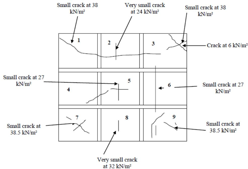
Figure 2. A scheme of the cracks before collapse, wall 4
