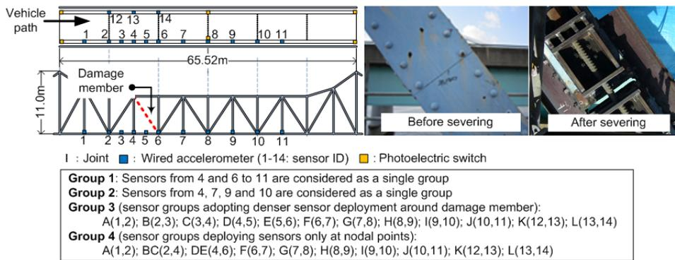
Figure 2. Sensor deploying map and damaged member.
