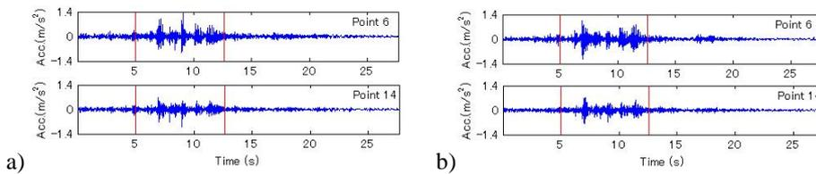
Figure 3. Vehicle-induced vibrations: a) Healthy ( $v=40$  km/h, Run3); b) Damage ( $v=40$  km/h, Run3).
