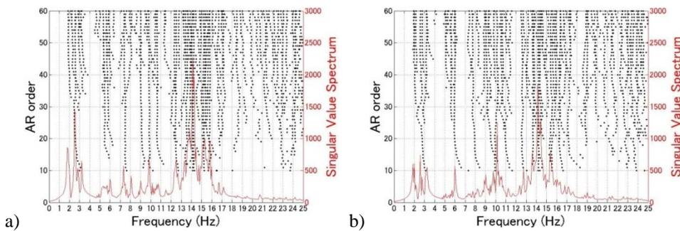
Figure 4. Stabilization diagram from vehicle-induced vibration data: a) Healthy ( $v=40$  km/h, Run3); b) Damage ( $v=40$  km/h, Run3).
