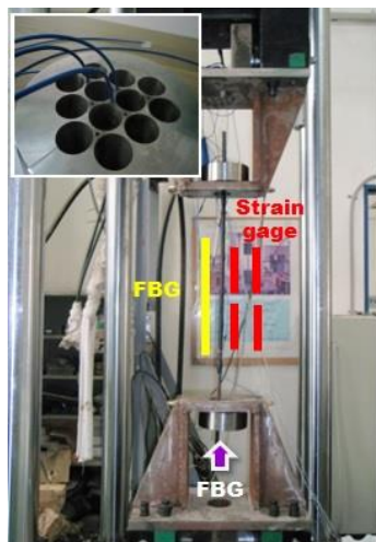
Figure 10. Tension test for PS strand and anchor head.
