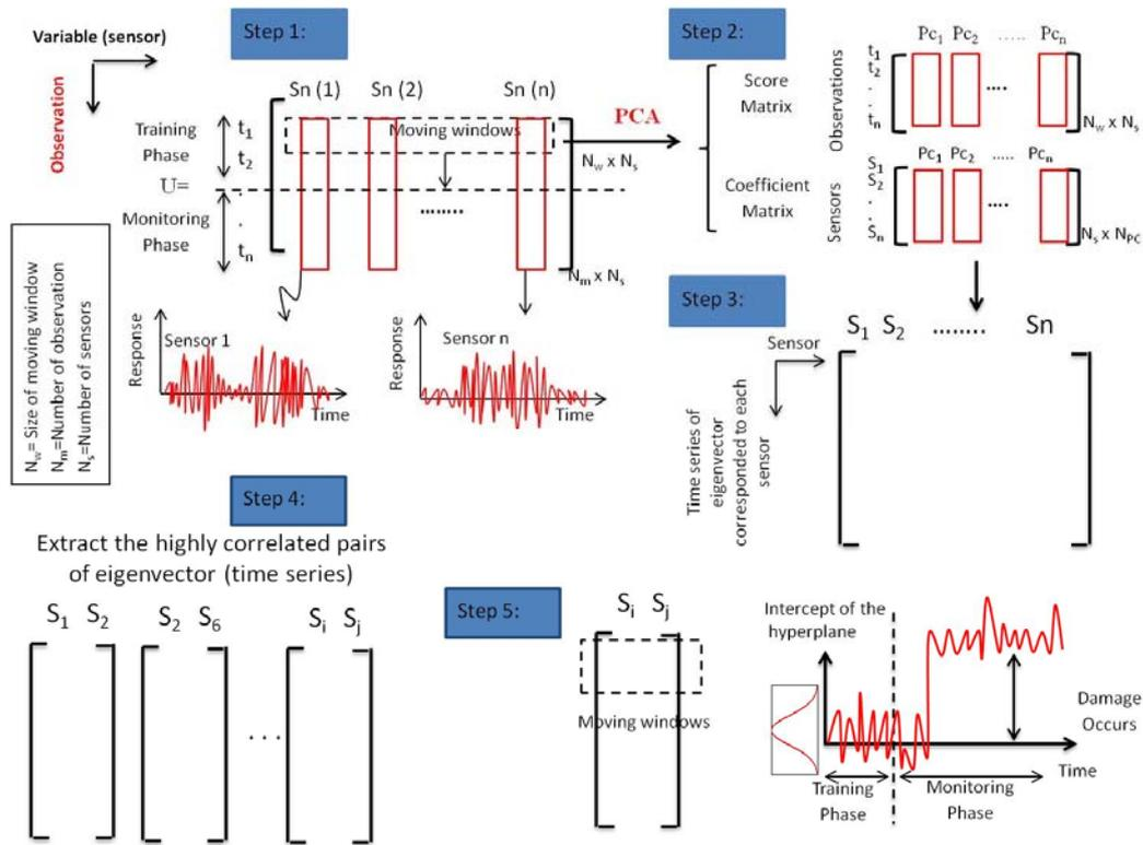
Figure 2- Procedures for long term SHM using MPCA-SVM algorithm
