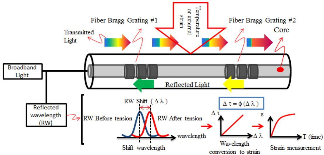
Figure 1-Measurement principal of Fiber Bragg Grating (FBG) sensor
