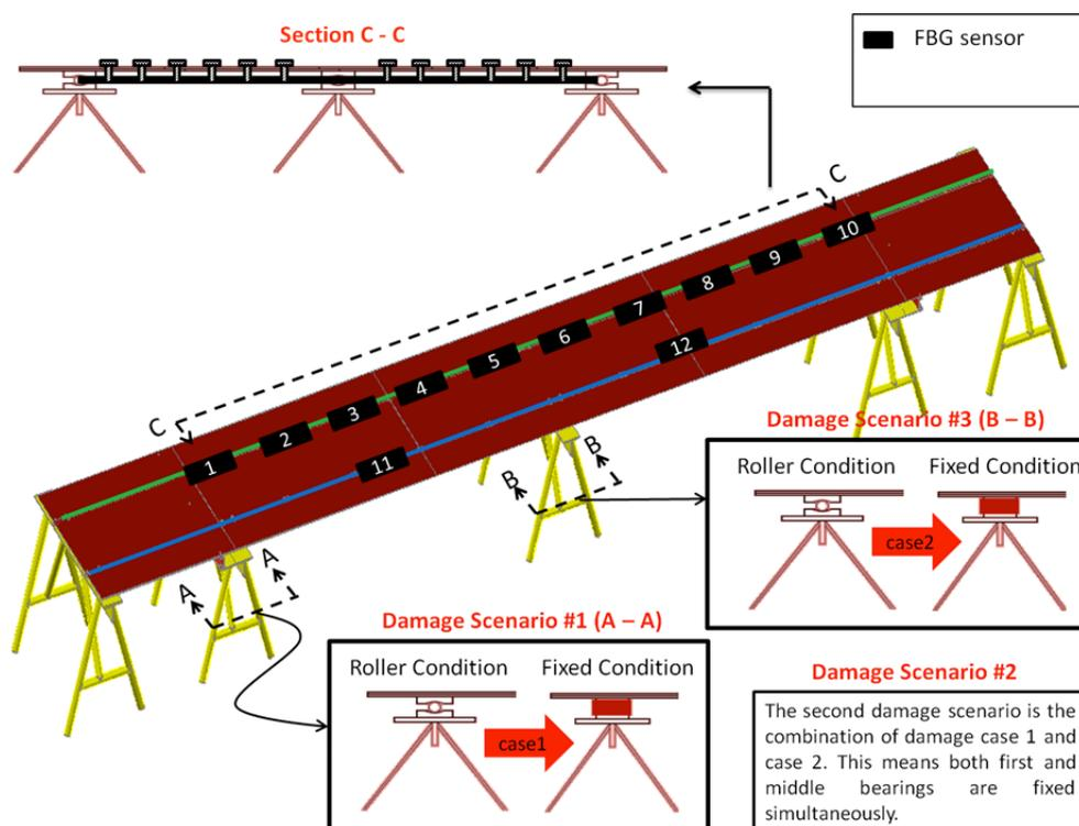
Figure 3- Location of sensors and simulated damage (UCF 4-span Bridge)
