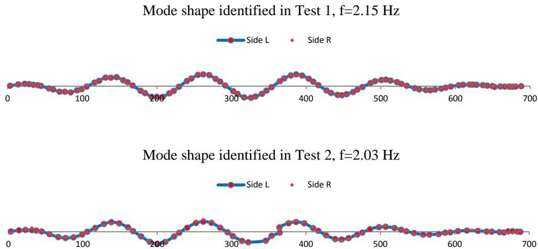
Figure 6. Mode shapes for the first vertical mode
