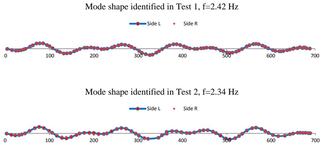
Figure 7. Mode shapes for the second vertical mode
