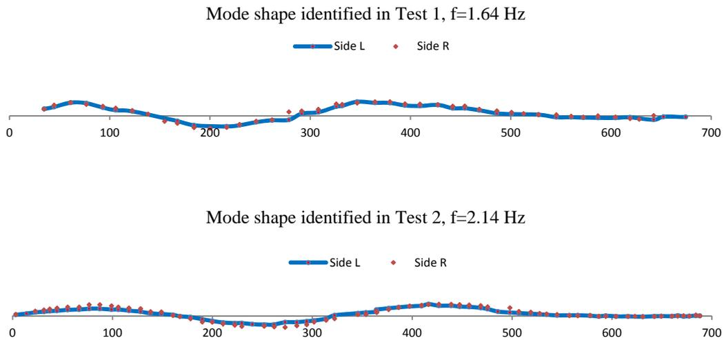
Figure 4. Mode shapes for the first transverse mode
