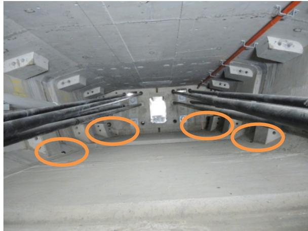
Figure 3. Accelerometers inside bridge girder in Test 2
