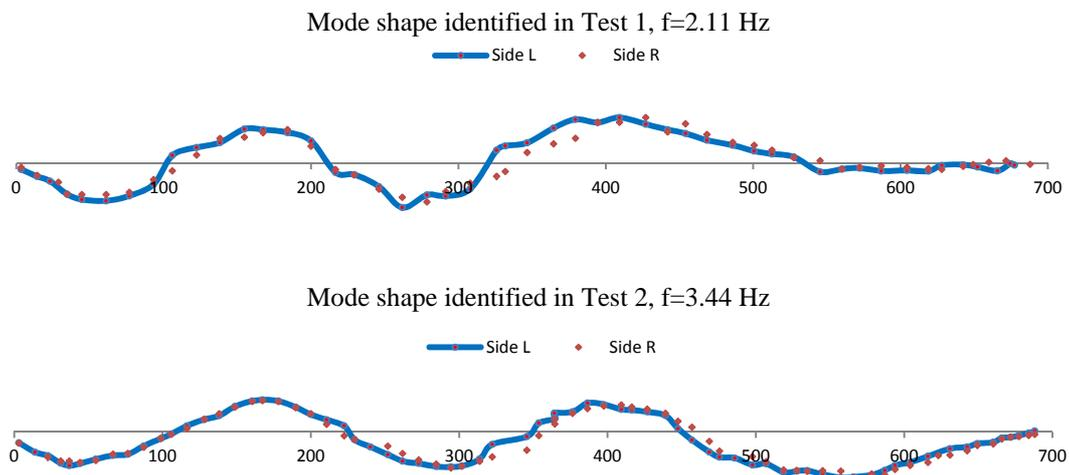
Figure 5. Mode shapes for the second transverse mode
