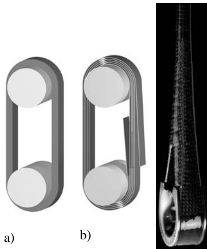
Figure 10. Conceptual design of pin-loaded strap elements.
