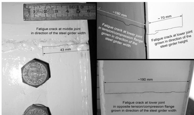
Figure 3. Fatigue cracks in welds after 19 months of service
