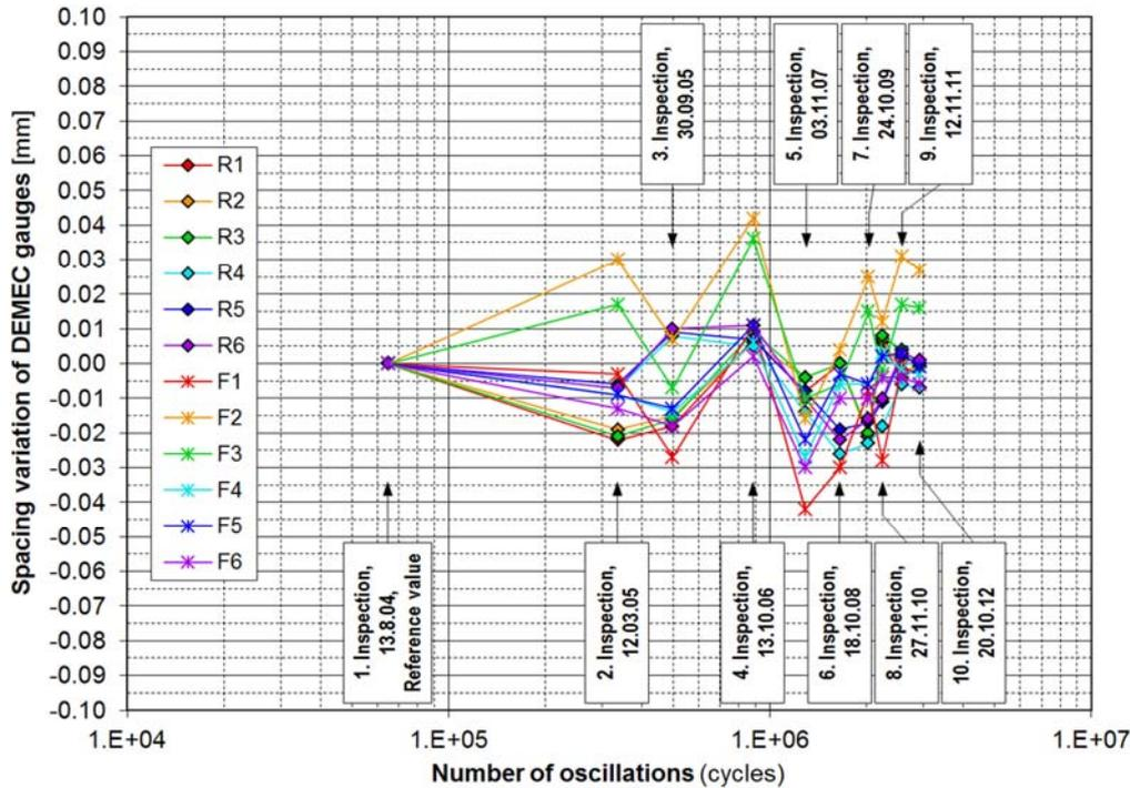
Figure 7. Spacing variation of DEMEC gauge as a function of the number of oscillations
