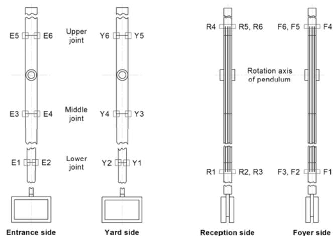
Figure 5. Six prestressed CFRP laminates bonded on the flanges of the artwork pendulum
