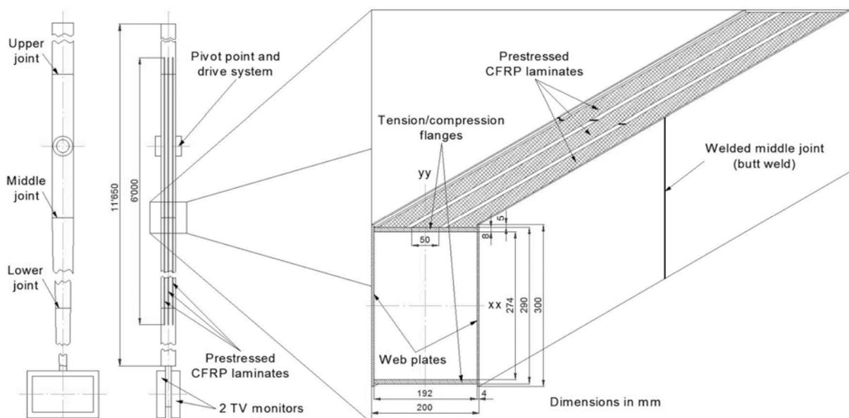
Figure 4. Strengthening principle of welds in the steel box girder; Details at middle joint
