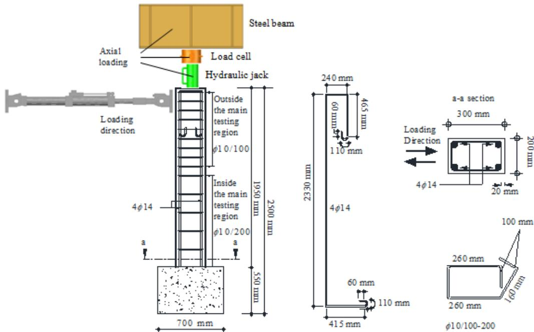
Figure 1. The geometry and reinforcement details of the tested columns.
