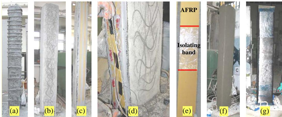
Figure 3. a) Removal of cover concrete, b) Application of a thin layer of cement based structural repair mortar to obtain a flat surface, c) Installation of the AFRP pultruded laminates (the specimen LAM), d) Application of additional AFRP laminate anchorages (only for the specimen LAM-LAM), e) Wrapping with a plastic isolating band (only for the specimen LAM-PB), f) Application of last layer of structural repair mortar, g) Wrapping with CFRP sheets in transverse direction.
