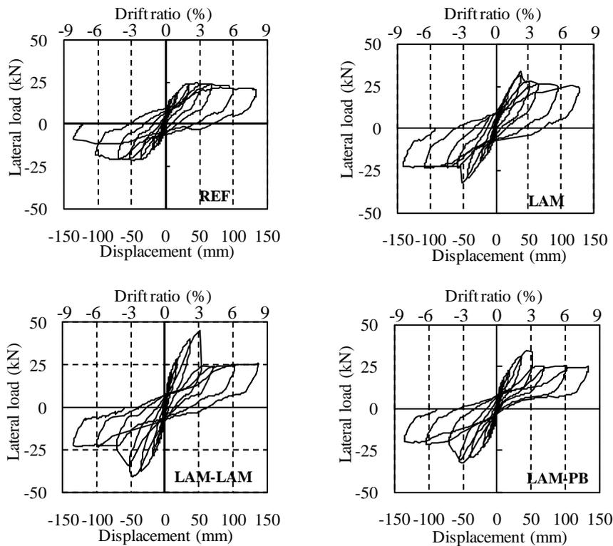
Figure 4. Lateral load-displacement curves for all specimens.
