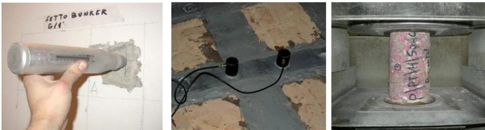
Figure 4. Material testing: (a) Rebound hammer; (b) Ultrasonic survey; (c) Concrete core testing.
