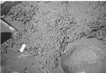
Figure 3 (a) Concrete mix with high W/C ratio
