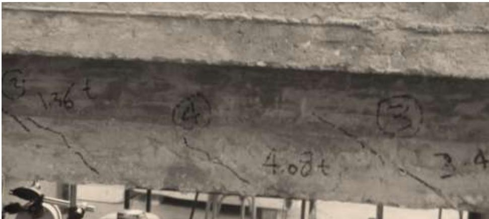
Figure 7: Failure mode of beam LB3
