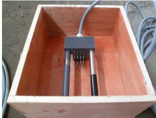
Fig-1: Sensor probe fixed in a wooden mould before pouring concrete
