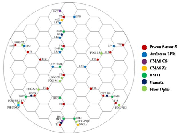
Figure. 2. A schematic drawing of cable cross section showing the embedded Precon temperature/humidity sensors and LPR/CMAS corrosion sensors and their distribution
