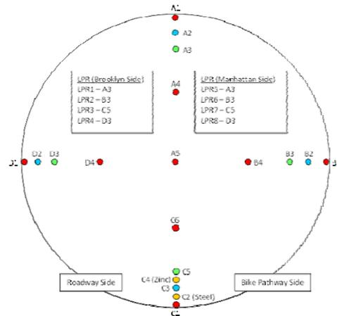
Fig. 8. Sensor distribution diagram within the cross section of the main cable.( grooves A,B,C &D) where A1, A4 and A5 are temperature/humidity sensors and A2 and A3 are corrosion sensors.
