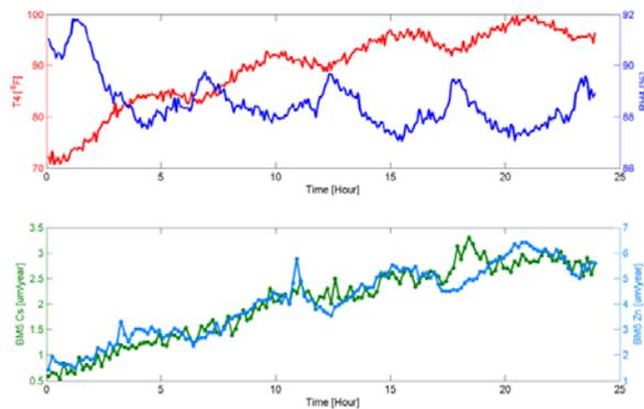
Fig 5. A direct data plot of temperature /humidity internal sensor (top) and corrosion bimetallic sensor (bottom) showing direct correlation between temperature, humidity and corrosion rate.
