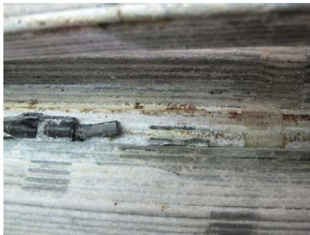
Fig. 6. View of cable mockup during the after completing the test showing a temperature, humidity sensors which survived the harsh environmental test and compaction.
