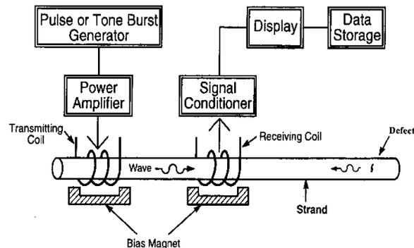
Fig 7. Magnetostrictive sensors system diagram
