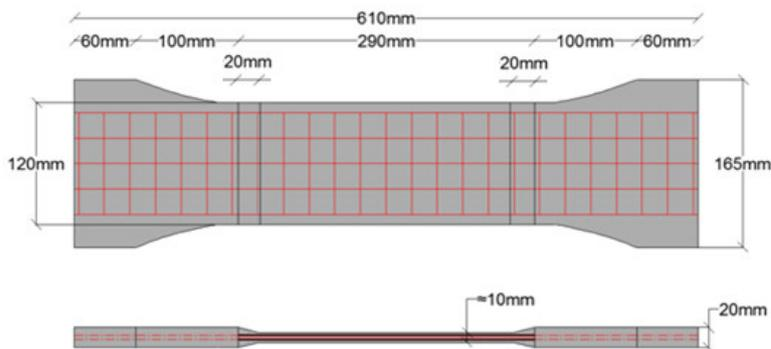
Figure 1. Configuration of coupons (Triantafillou 2012a).
