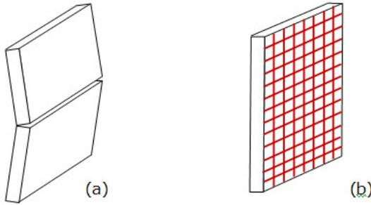
Figure 3. (a) Vertical flexural failure, (b) strengthening by TRM System (Triantafillou 2012b).
