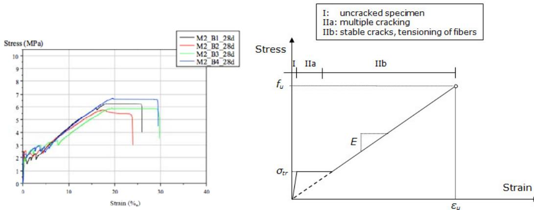
Figure 2. Left: Real stress-strain behaviour of the coupons constructed with Basalt fabric and C-Matrix Type F mortar, Right: Simplified stress - strain curve of TRM System (Triantafillou 2012a)
