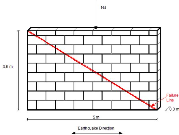
Figure 4. Wall subjected to in-plane load
