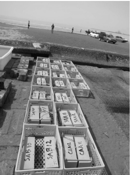
Figure 2. Small beams located in tidal zone of the field exposure station.
